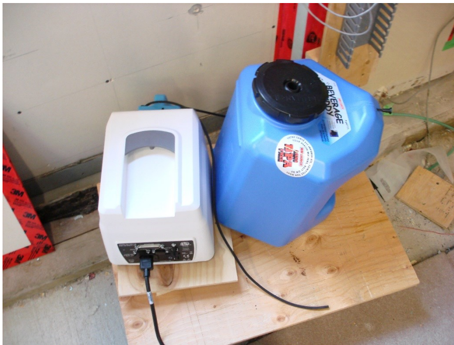
Figure A. 1. Cole-Parmer Masterflex® L/S® peristaltic pump and a water container used to calibrate the wall rain gauges and leakage gauges.
