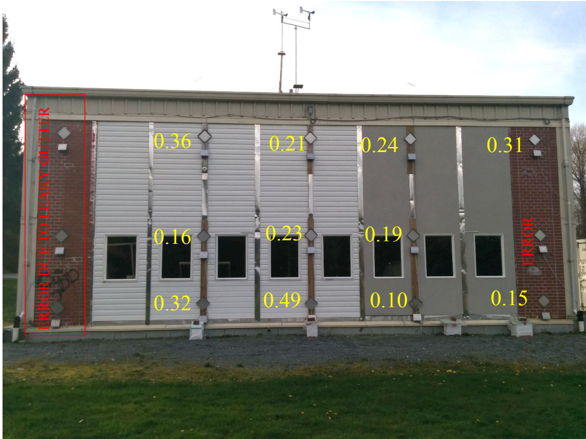
Figure 40. Rain Admittance Factors (numbers in yellow) calculated based on the measured WDR at the respective wall rain gauges and the free-field WDR as calculated following the Straube and Burnett’s method.
