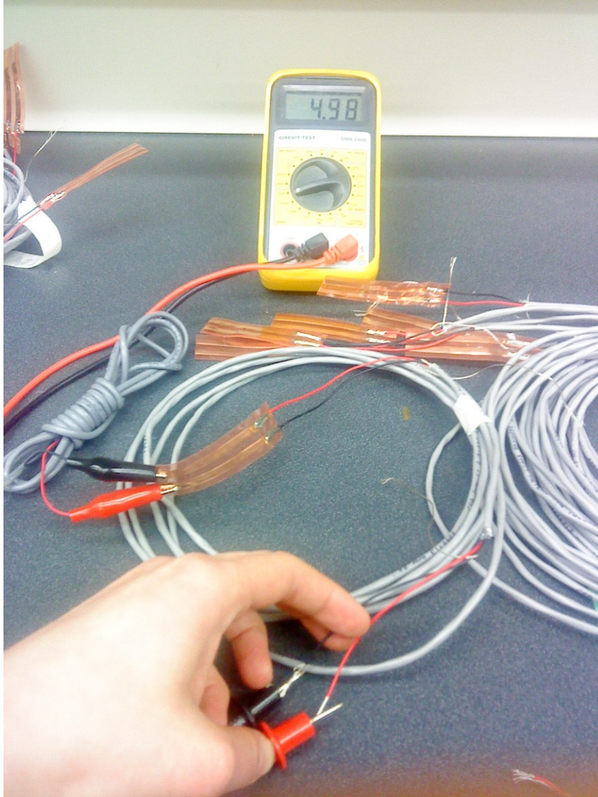
Figure A. 6. Testing setup for moisture detection tapes.
