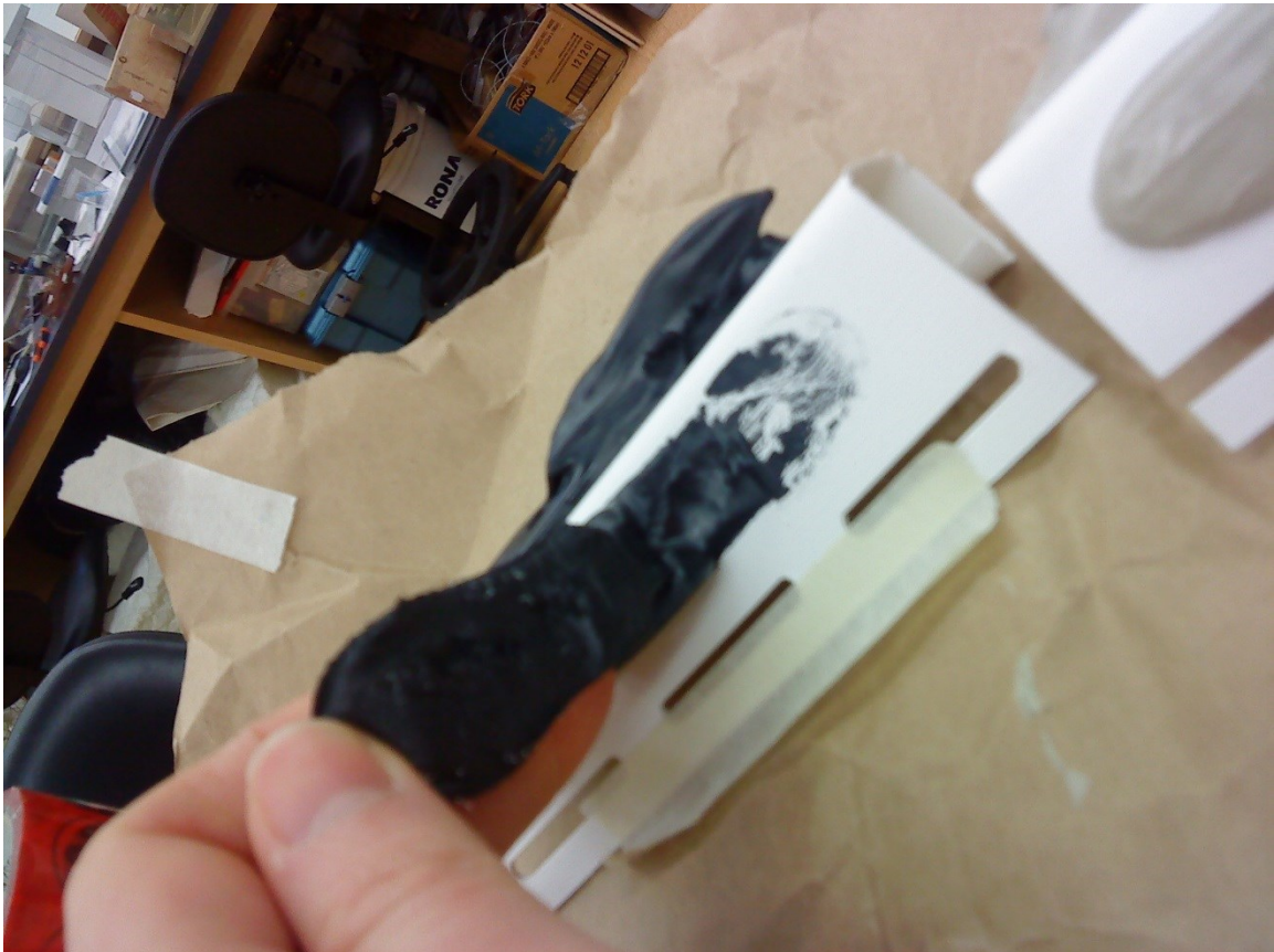
Figure 11. LePage Quad Advanced Formula exterior sealant passed the adhesion pull test on a vinyl siding J-trim as the sealant showed cohesive failure, instead of adhesive failure when pulled away from the substrate.
