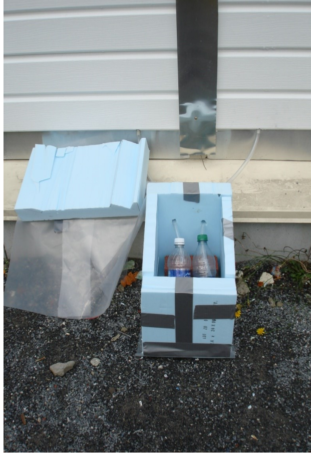
Figure 30. XPS housing for the bottles collecting drainage water from W3 and W5 vinyl siding walls.
