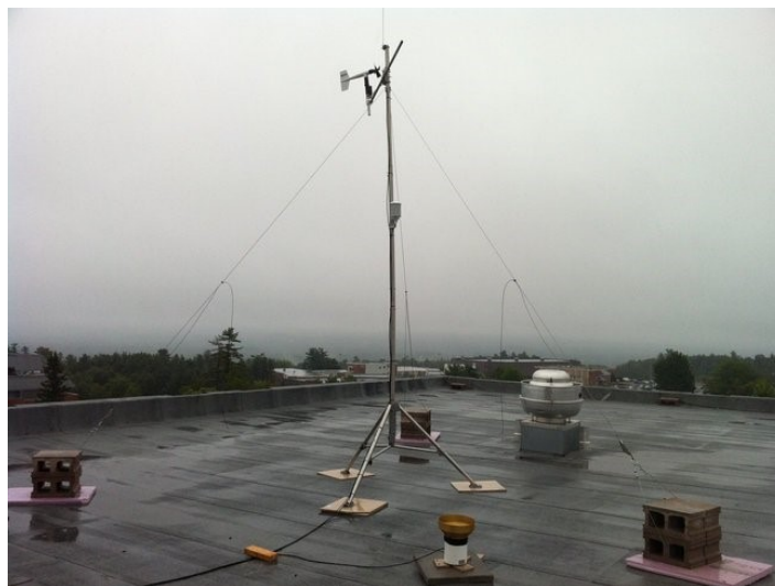
Figure 3.3: Photo of wind monitor, temperature and relative humidity probe and the horizontal rain gauge installed on the roof top of McLeod House
