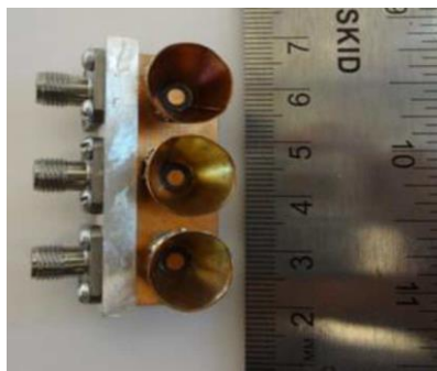
(c) Triple Hybrid microstrip antenna sensor [59].
