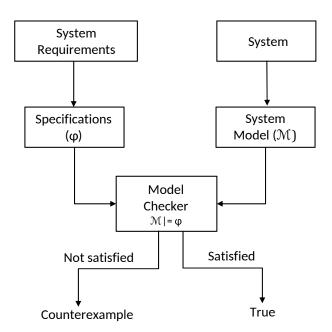
Figure 2.2: A typical model checker
