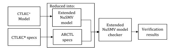
Figure 5.2: Reduction technique workflow
