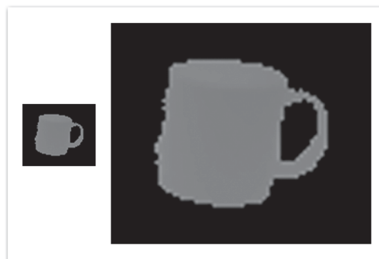
FIGURE 3.14: Left: original depth image patch. Right: scaled depth image patch.
