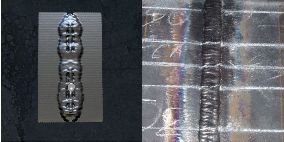
Figure 33: The left image is the simulation result of our system. The right image is a photo of welding.
