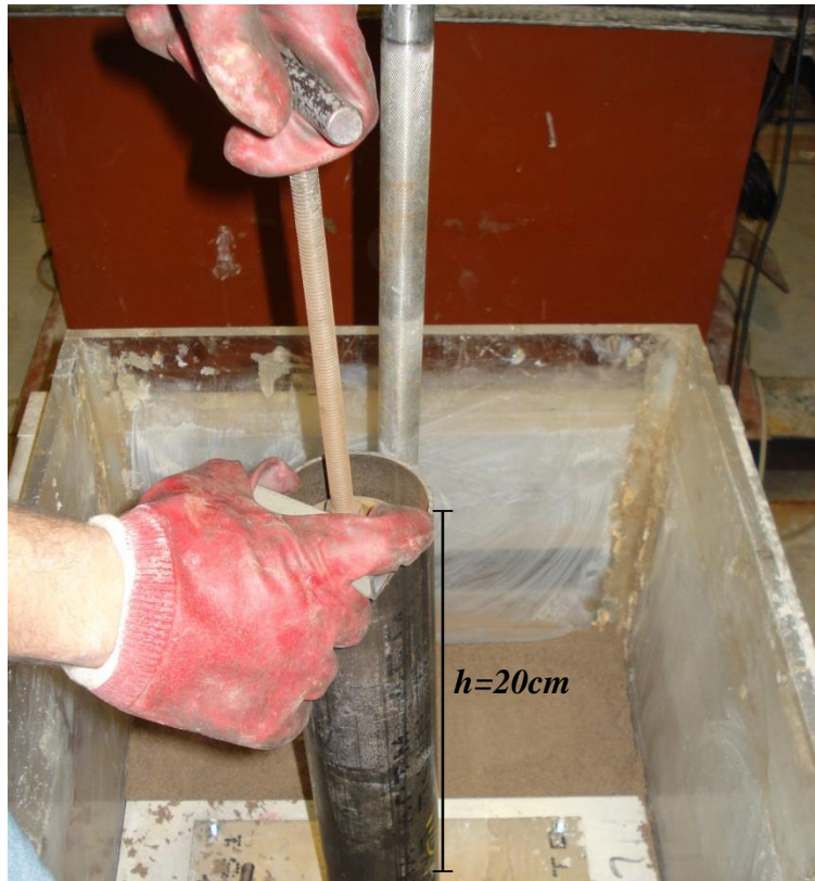
Figure 3.22 Compaction in soil tank
