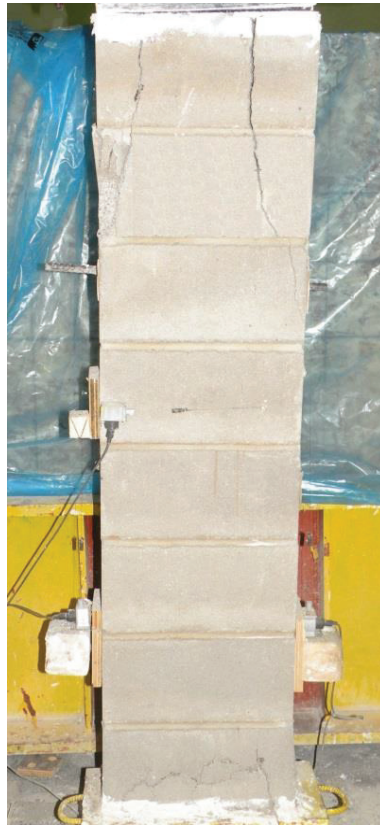
Figure 3.24: Typical failure mode for URM prisms in group G4-P8S with h/t equal to 8
