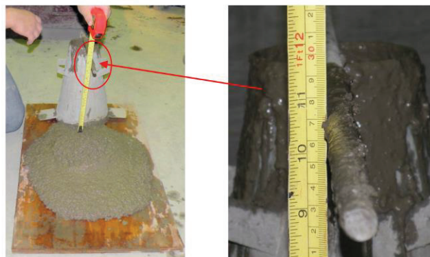
Figure 3.12: Slump test for grout
