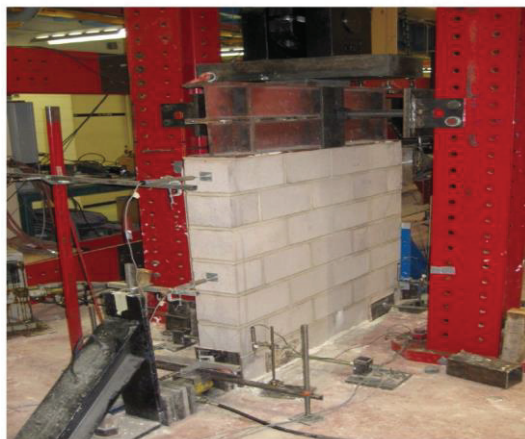
Figure 2.14: Test setup for PG masonry walls (Oan and Shrive, 2012)
