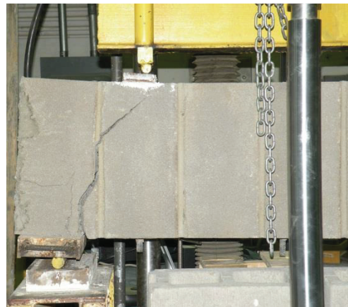
Figure 3.32: In-plane beam shear test: (a) test setup; (b) typical mode of failure
