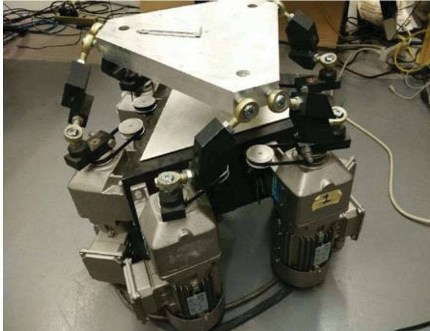
Figure 2.4: 6-RSS parallel robot
