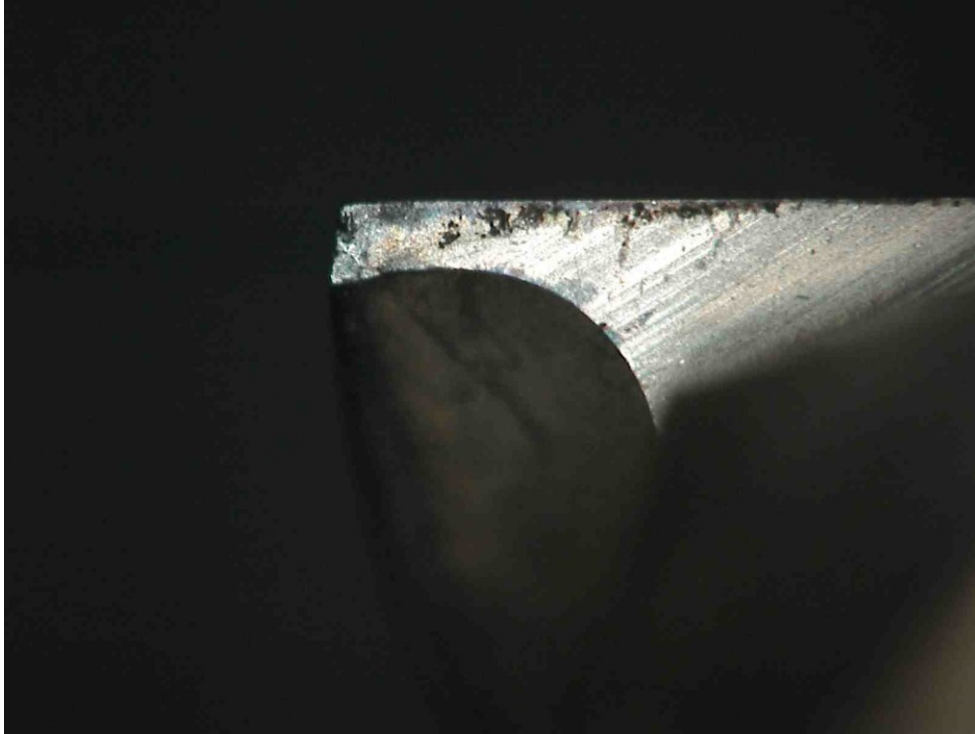
Figure 1.3 Chipping of the edge on a flat end-mill
