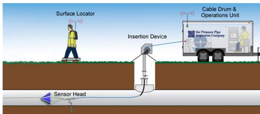
Figure 2-5.Sahara leak detection technique (adopted from [www.puretechltd.com](http://www.puretechltd.com))
