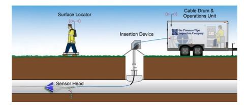
Figure 2-5.Sahara leak detection technique (adopted from www.puretechltd.com)
