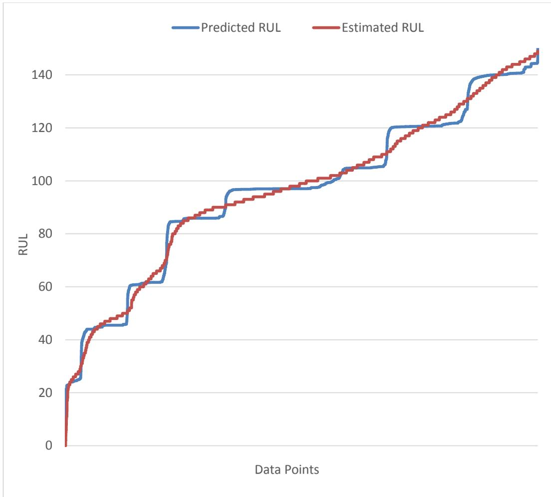
Figure 5-21. Estimated and Predicted RUL vs data points using LM algorithm
