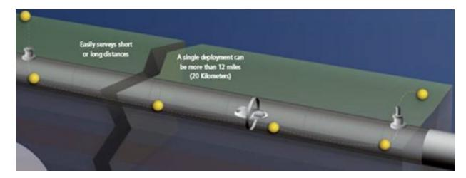
Figure 2-7.Smartball deployment and recovery (adopted from rebar.ecn.purdue.edu)
