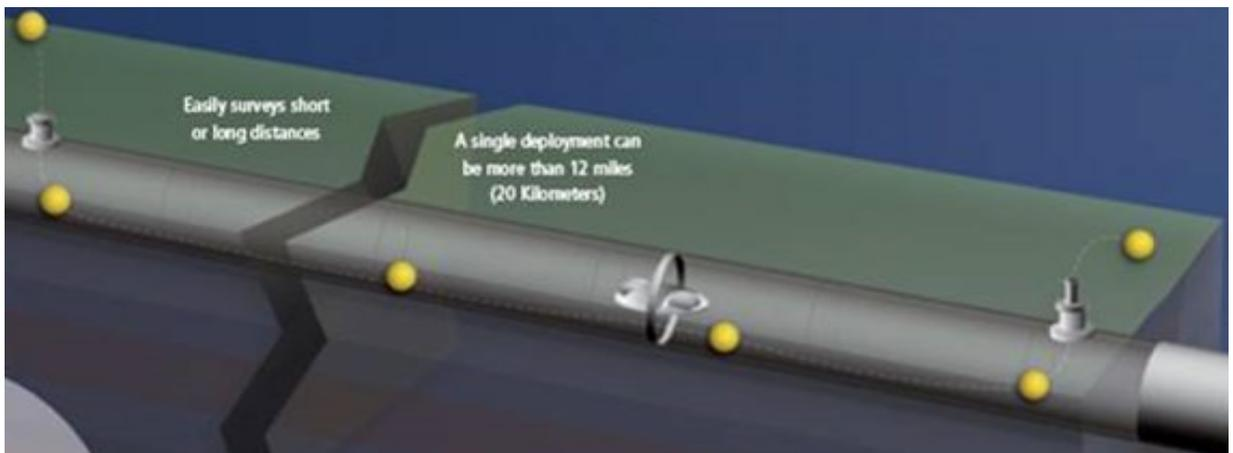
Figure 2-7. Smartball deployment and recovery (adopted from rebar.ecn.purdue.edu)
