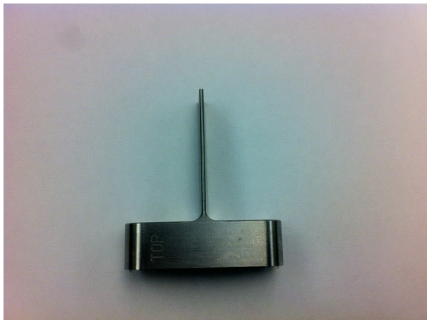
Figure B-2: Airfoil Ti-6Al-4V sample geometry with dimensions in mm.
