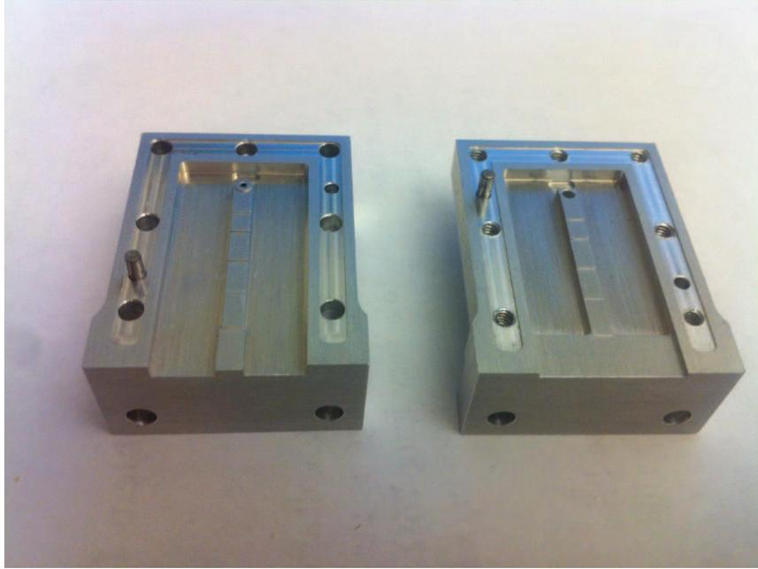
Figure 2.14: The internal configuration of the fabricated connector.
