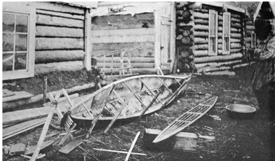
Fig 2.11 Canoe from Lower Yukon with rigid floor frame. Reprinted from Adney, T. & Chapelle, H. (1964) The Bark Canoes and Skin Boats of North America . Washington D.C.: Smithsonian Institute, 165.
