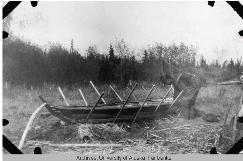
Caption Fig. 2.7 “Below is shown the next step. The large sheets of birch bark are pinned in position with wooden pins and the ribs are also placed.”
