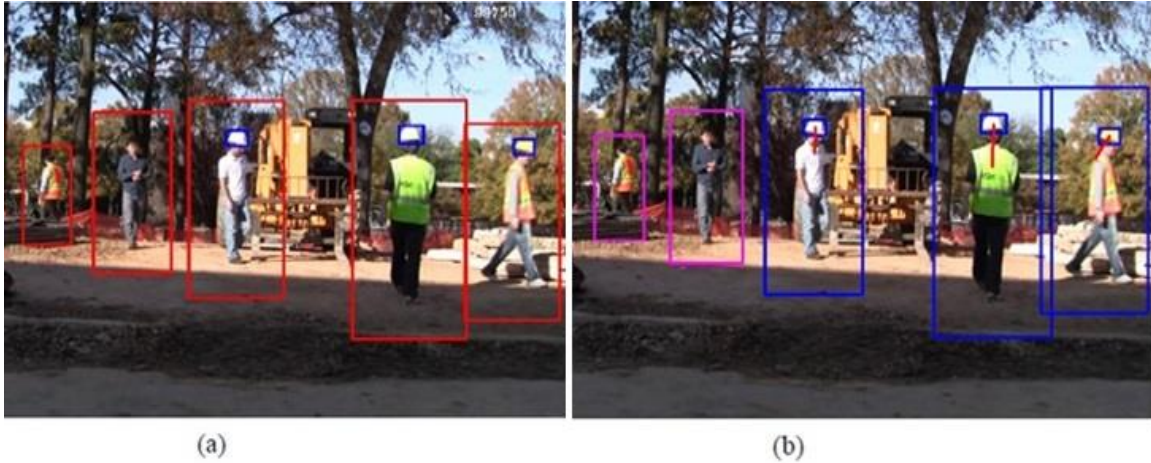
450 Figure 3-13: Example of the HOG-based detection and matching (a) Human body 451 and hardhat detection. (b) Matching between the detection results.
