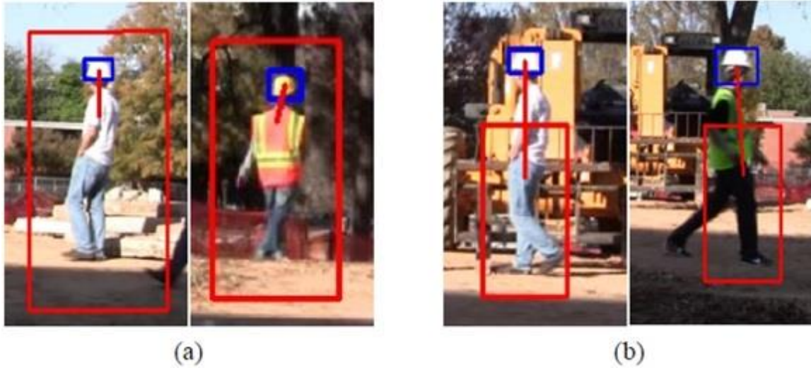
479 Figure 3-15: Matching between the human body and hardhats. (a) Matching in 480 Region I. (b) Matching in Region II.
