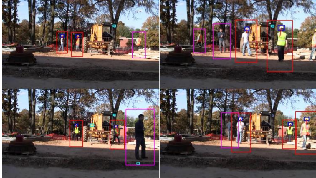
Figure 4-5: Examples of identifying people with hardhats (red) and without hardhats (magenta).
