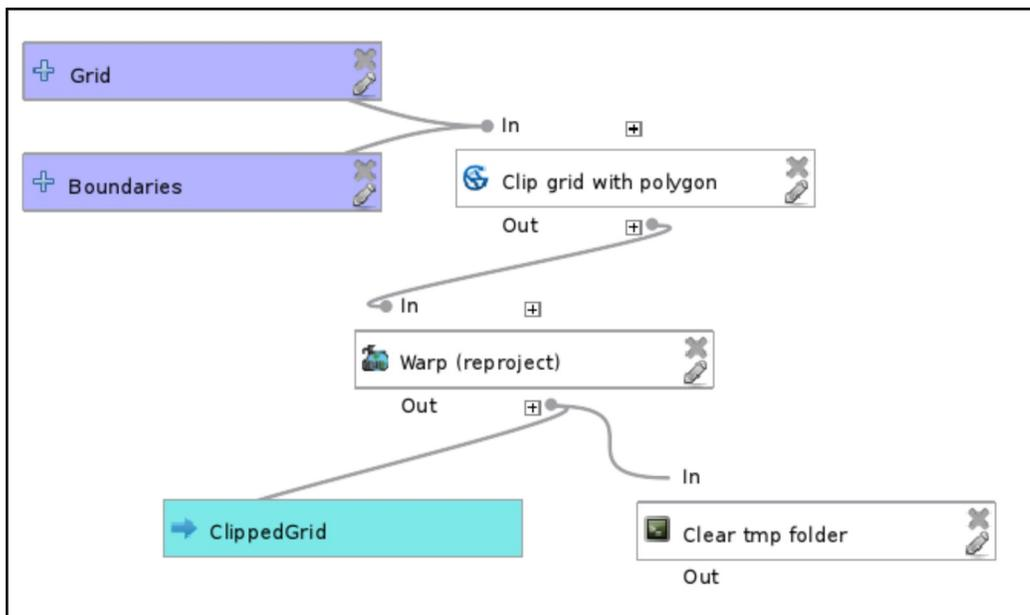
Figure 7-1: QGIS Graphical Model for Batch Clipping and Warping Raster Grids
