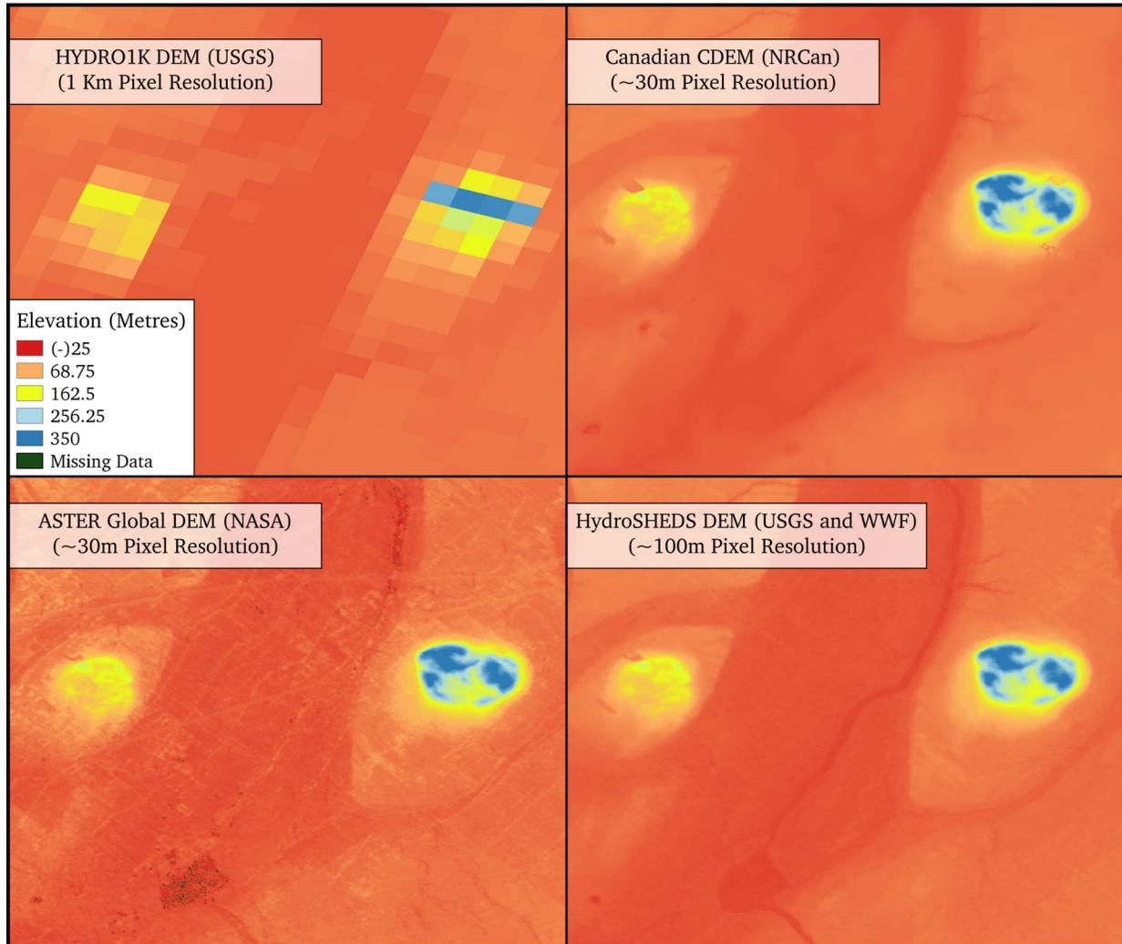
*Figure 7-2: Comparison of Different Elevation Models showing Resolution differences and Artifacts*
