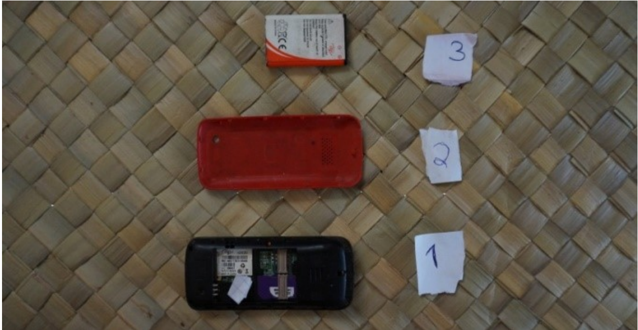
Figure 66: 1. Interior of Mobile Phone. 2. Back plate. 3. Battery, Gwou'ulu, September 2014 © Geoffrey & Stephanie Hobbis
