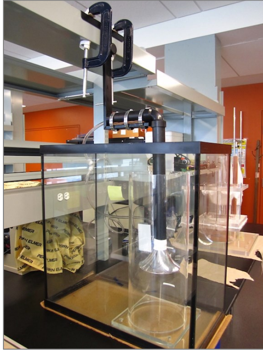
Figure 4.2 Reactor with a Plexiglas cylinder and air jet arm connected to the central air compressor.
