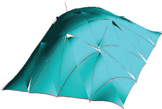
Figure 7.3: A surface over a 64-element mesh. Each element has 1 collocation point and 2 matching points per edge.
