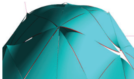
Figure 7.4: A zoomed-in view of the surface for showing the shapes of the patches and the gaps between each pair of adjacent patches.
