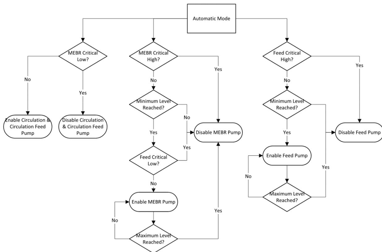
Figure 5.2-1: Pump Controller – Automatic Mode
