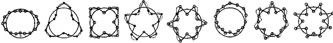
Figure 1.14: The first eight mode shapes of radial resonance obtained using experimental modal analysis by Yam et al. [114]
