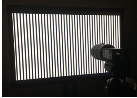
Figure 17: Phase-Shifting camera calibration set-up
