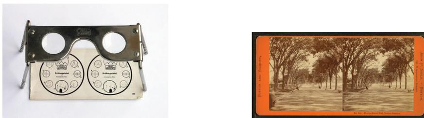
Figure 1: Left image is a pocket stereoscope with original test image. Used by military to examine stereoscopic pairs of aerial photographs. Right image is a view of Boston, c. 1860; an early stereoscopic card for viewing a scene from nature.
