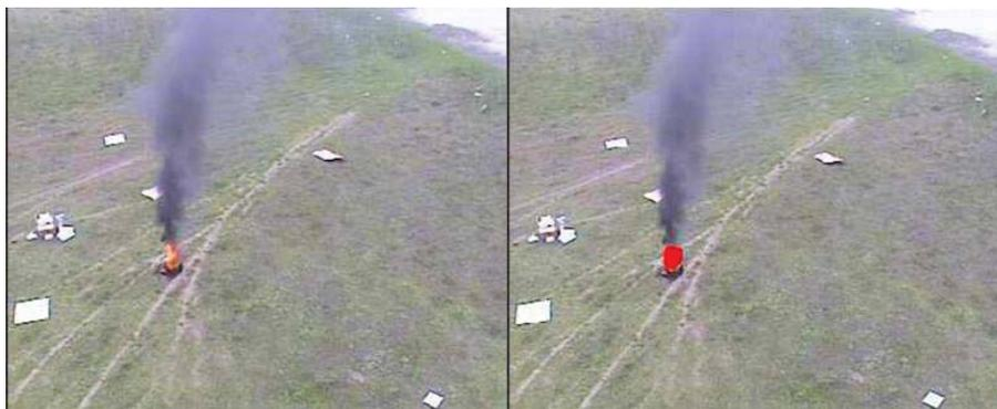
Figure 2.1: Segmentation of visual image: original (left) and segmented (right) images [2].
