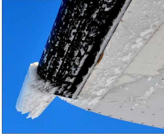
*Figure 1-3: Rime ice left-over on a wing leading edge after de-icing boot (black component) activation [9]*
