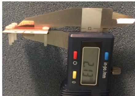
Fig. 3-2. Measuring the thickness of stacked layers with regular plastic screws to identify possible gap height between them.
