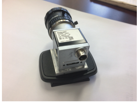
Figure 2.3: The High speed camera used to record the trajectory of the spheres
