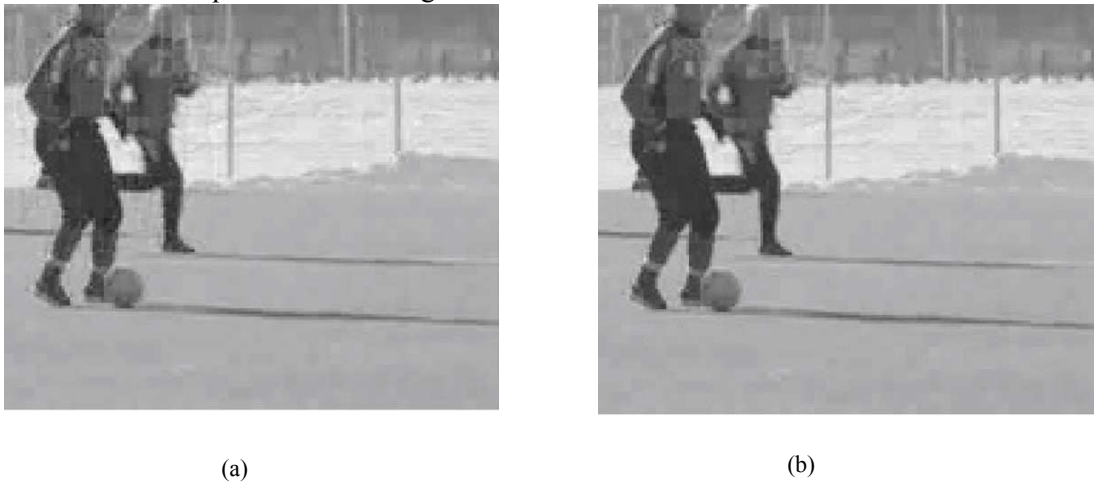
Figure. 3.17: 47th decoded frame of the Foreman sequence, (GOP size :2 and quantization matrix Q6) (a) Decoded frame by the DISCOVER codec, PSNR=31.99 dB, number of bits required for decoding: 17086 bits. (b) Decoded frame by the modified DISCOVER codec, PSNR=32.6 dB, number of bits required for decoding:15575 bits
