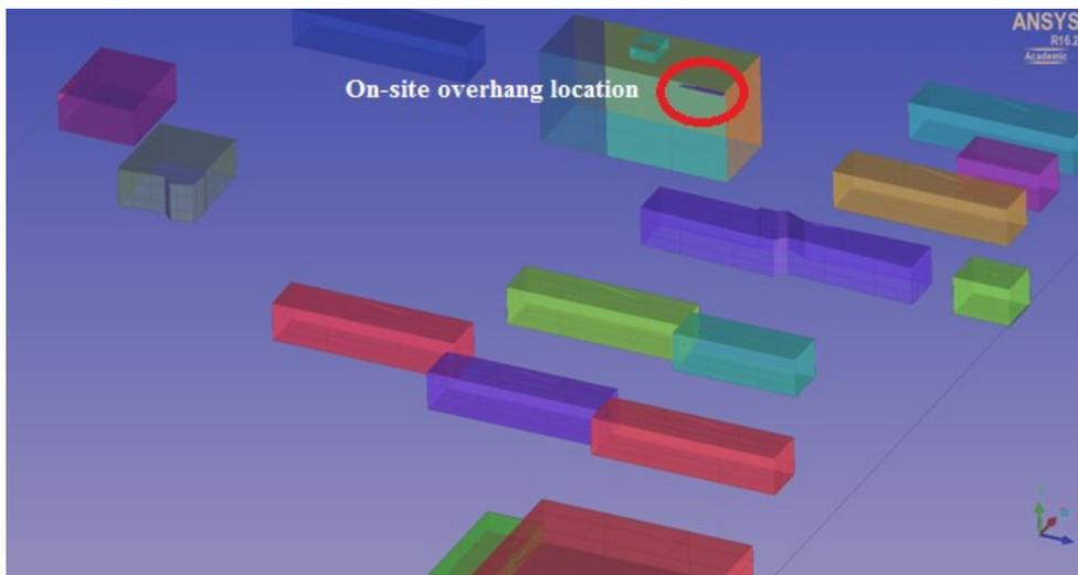
Figure 4.2.1 - The east façade at normal wind, surrounded by upwind buildings equipped with 4' on-site overhang
