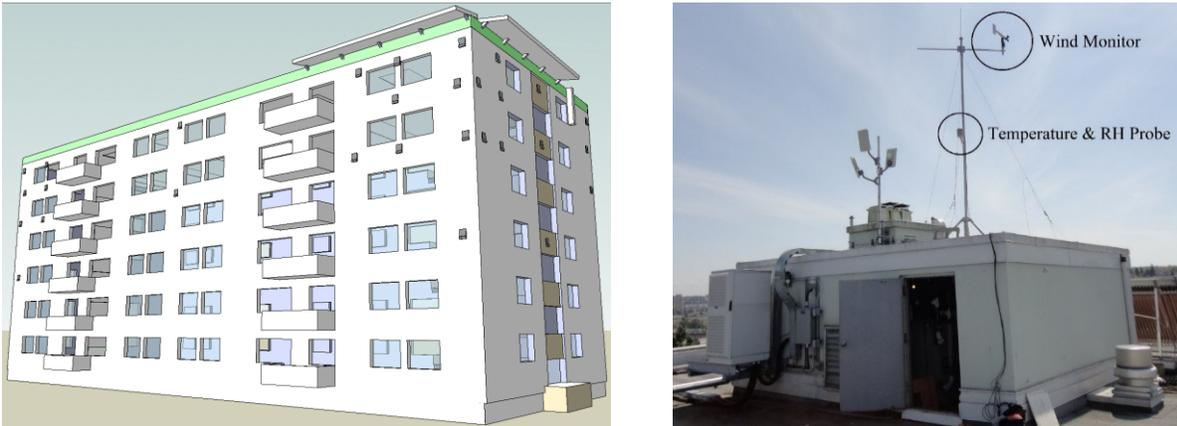
Figure 2.3.14 - Schematics of the building and the mechanical room with the wind monitor mounted on top of it (Chiu, 2016)
