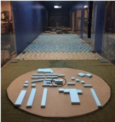
Figure 2.3.11 - The test building and surrounding buildings within a 200-m radius placed in ABL wind tunnel (Chiu, 2016).
