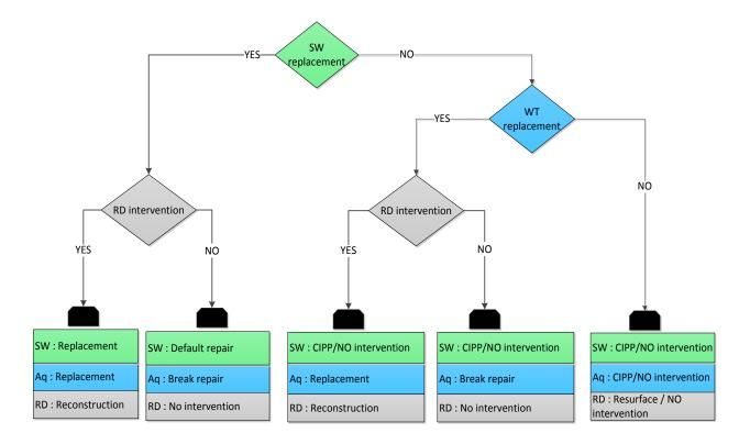
Figure 3.9 : Scenario 2 – Water or sewer pipe replacement if road is reconstructed
