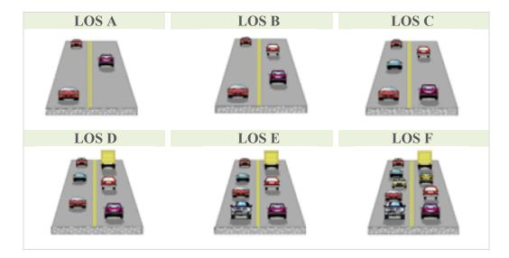
Figure 5.4 : Level of service for road segments (Courtesy of Montreal Polytechnic School)
