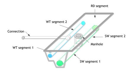
Figure 3.7 : Example of a typical trench
