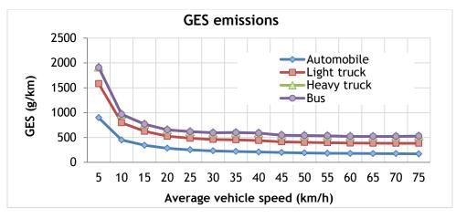
FIGURE D1: GES emissions-speed curve (MTQ, 2013)
