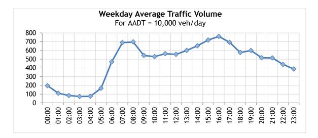
Figure 5.3 : Montreal traffic volume pattern per the time of the day (City of Montreal)
