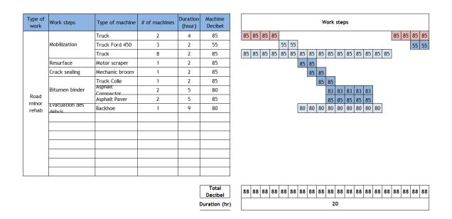
Figure 5.11 : Noise duration diagram for road minor rehabilitation
