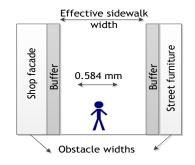
Figure 5.6 : Effective width on a sidewalk (Finch, 2010)
