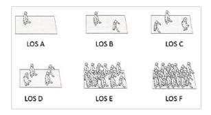
Figure 5.7 : Levels of service for sidewalks (HCM, 2000)
