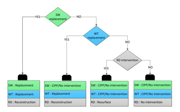
Figure 3.8 : Scenario 1 - Road reconstruction if water or sewer pipe is replaced
