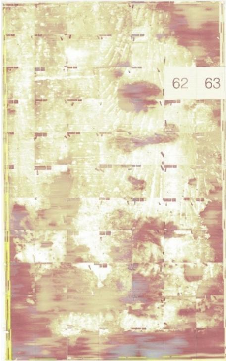
Figure 4.2: The defective areas in the fused image without image processing
