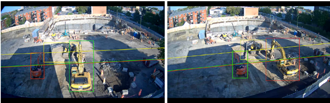
Figure 2.4 Object matching with epipolar lines
