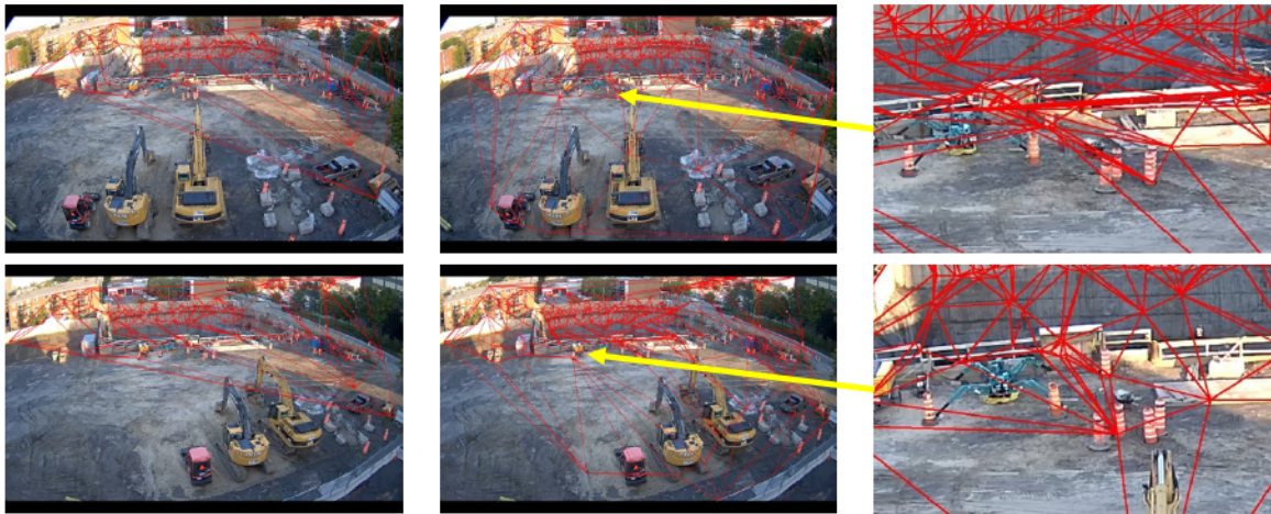
Figure 4.15 Triangle meshes generated by different thresholds
