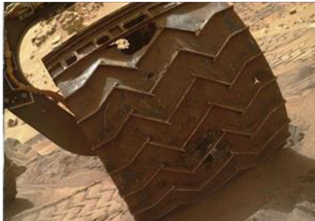
Figure 1-4: Tear and Punctures in Curiosity’s wheel Courtesy NASA/JPL-Caltech
