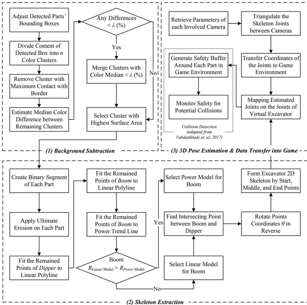
**Figure 6-1. Process of estimating 3D pose of excavator using stereo vision**
