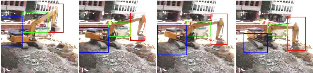
**Figure 5-22. Output of the parts' detection module**
