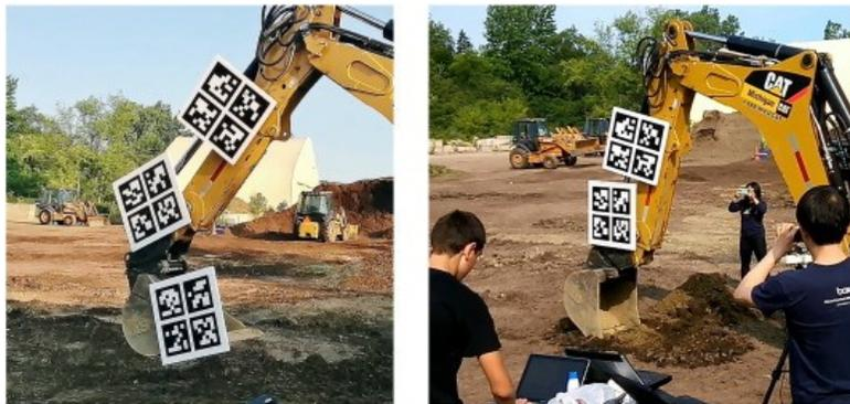
**Figure 2-8. Markers installed on backhoe (Lundeen, et al., 2016)**
