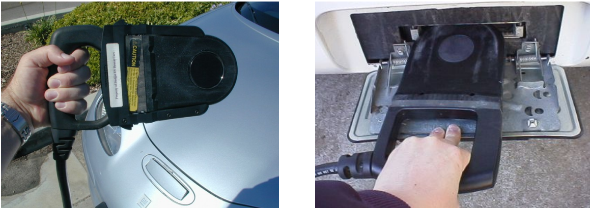
Fig. 1.1 Inductive charger paddle (left) and electric vehicle charging through the paddle (right) [7]
