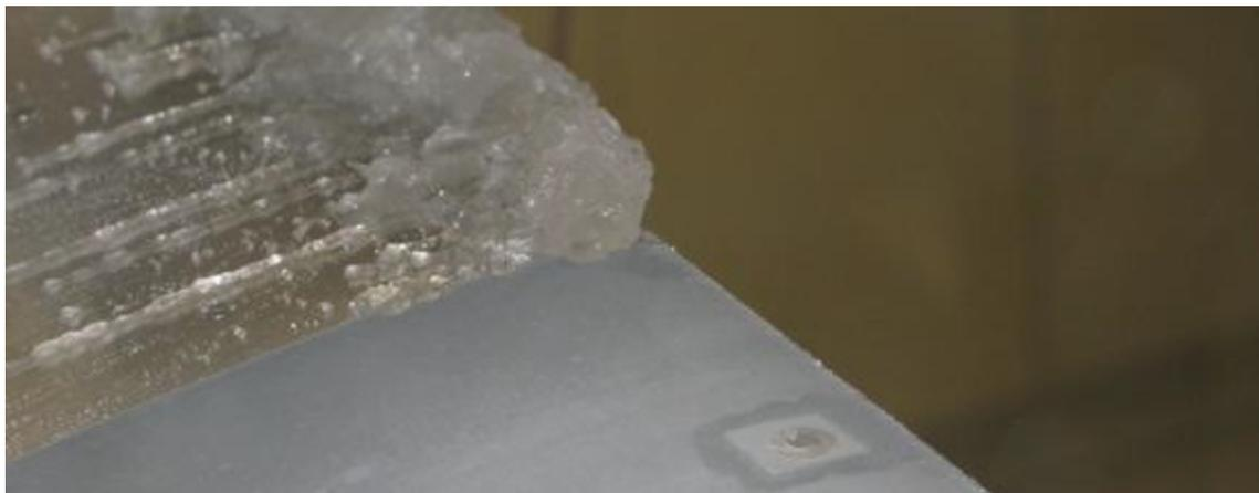
Figure 1.3. Comparison of a superhydrophobic surface (right/front) to a hydrophilic surface (left/back) in icing conditions<sup>1</sup>.
