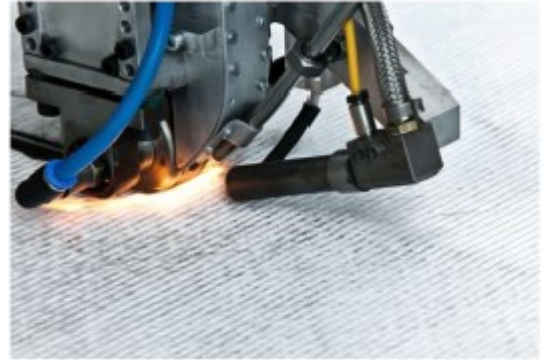
Figure 2.5: Schematic illustration of the DFP process (left), fiber placement head during DFP process (right) [31]
