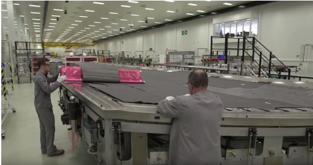
a) Operators placing NCF into mold
