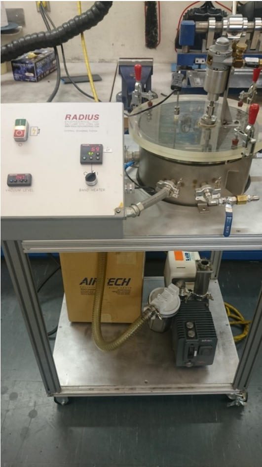
a) Resin degassing equipment
