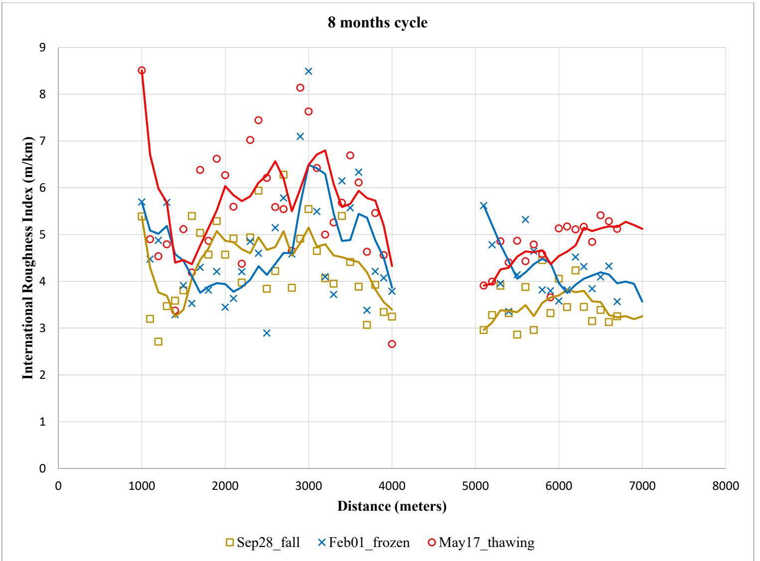
Figure 4-6 Clean Comparison of Pavement-surface roughness after removal of start/end and bridge sections.
