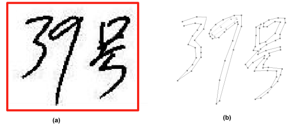
Fig. 4. Polygonization algorithm, (a) original handwriting images, and (b) polygonized contours.
