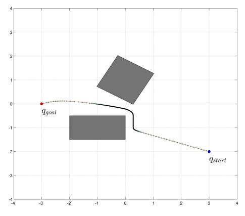
Figure 3.8: Planned path by updating  $\alpha$  at each iteration
