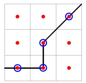
(a) A generic implementation of A\* only explores centers of cells and the f score is associated with the center of each cell
