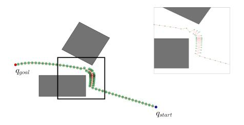
Figure 3.7: Planned path generated by simple integration with oscillations
