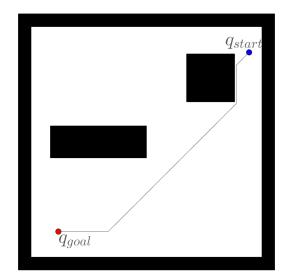
(a) A path found using gradient descent on the wave front grid
