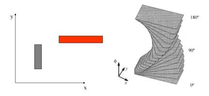
Figure 2.4: A configuration space with start and goal states of a rigid body [5]
