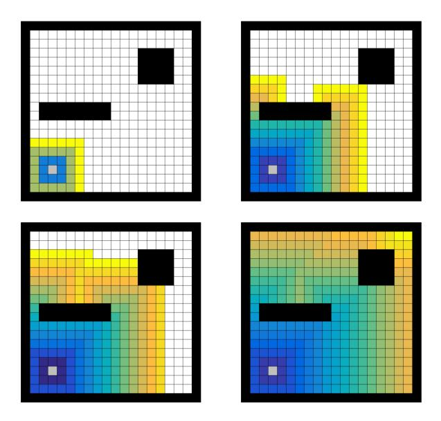
Figure 3.23: Wave front planner growing inside a workspace different colors represent different cost of a cell
