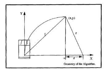
Figure 5.10: Geometry of Pure-Pursuit algorithm
