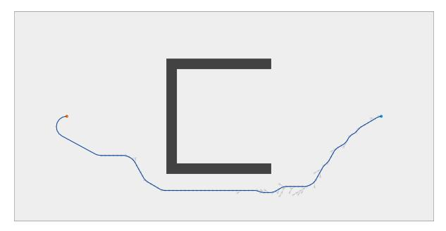
Figure 4.13: Unconstrained Heuristic, Visited Nodes: 107 Path Length: 7.617800 m
