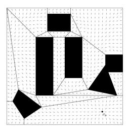
(a) A vector field is constructed directly without a potential function
