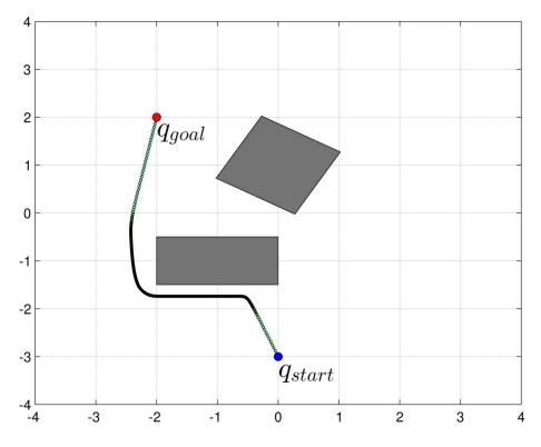
Figure 3.11: Planned path by updating  $\alpha$  at each iteration
