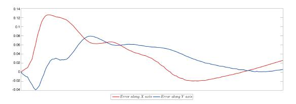
Figure 5.15: A depiction of cross-track errors along X & Y axes in (m) at configuration 2
