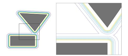
Figure 3.5: Equipotential contour of repulsive function around obstacles
