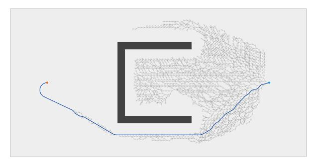
Figure 4.12: Constrained Dubins heuristic, visited nodes: 2213 Path Length: 7.408262 m
