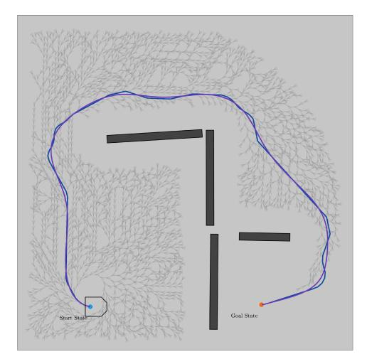
Figure 5.8: Hybrid A\* path vs a smooth hybrid A\* path
