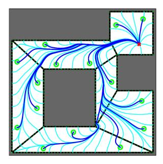
Figure 3.15: Choset et. al. [6] used the weak harmonic potential functions on decomposed cells
