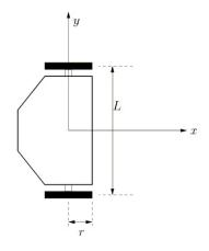
Figure 2.1: Geometry of a generic differentially driven robot [22]
