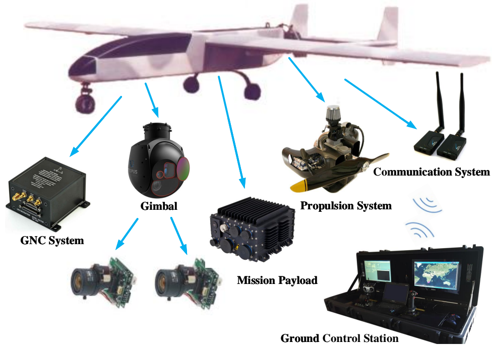
Figure 1.3: The fundamental architecture of a typical UAV system.
