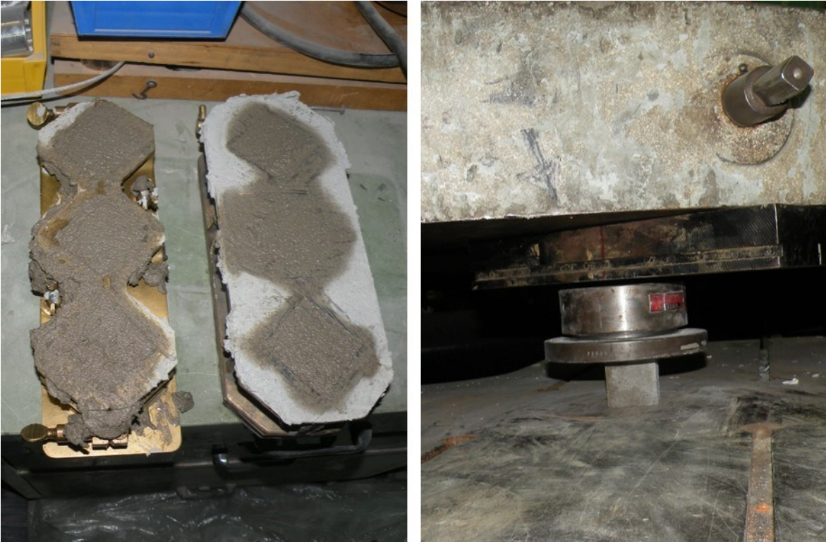
Figure A.4 Testing Type S mortar.
