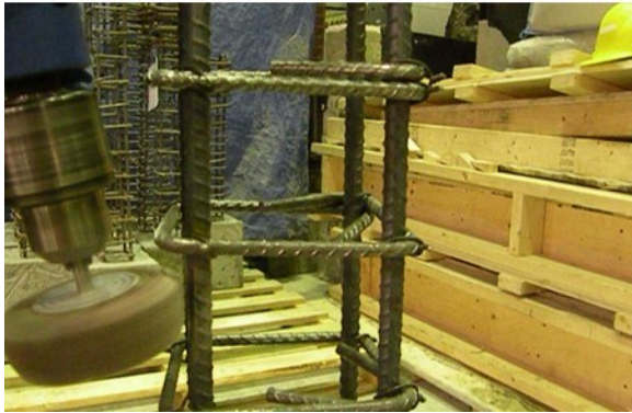
Figure A.19 Attaching strain gage to reinforcement steel.
