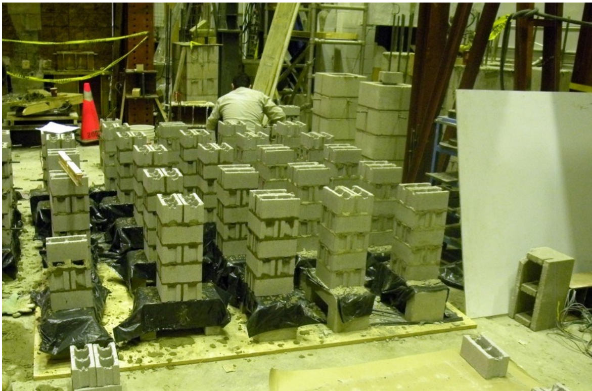
Figure A.3 Construction of concrete masonry prisms.
