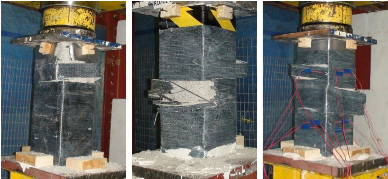
Figure C.6 Failure modes at the end of the compression tests for R10-L2.
