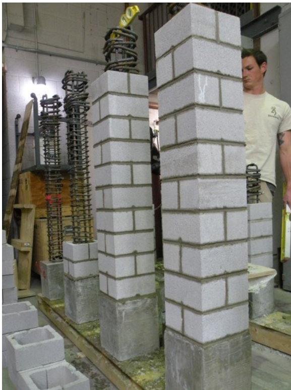
Figure A.20 Reinforced concrete masonry columns before grouting.
