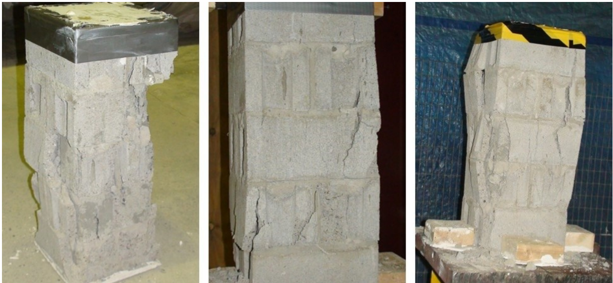
Figure C.2 Failure modes at the end of the compression tests for R0-L0.
