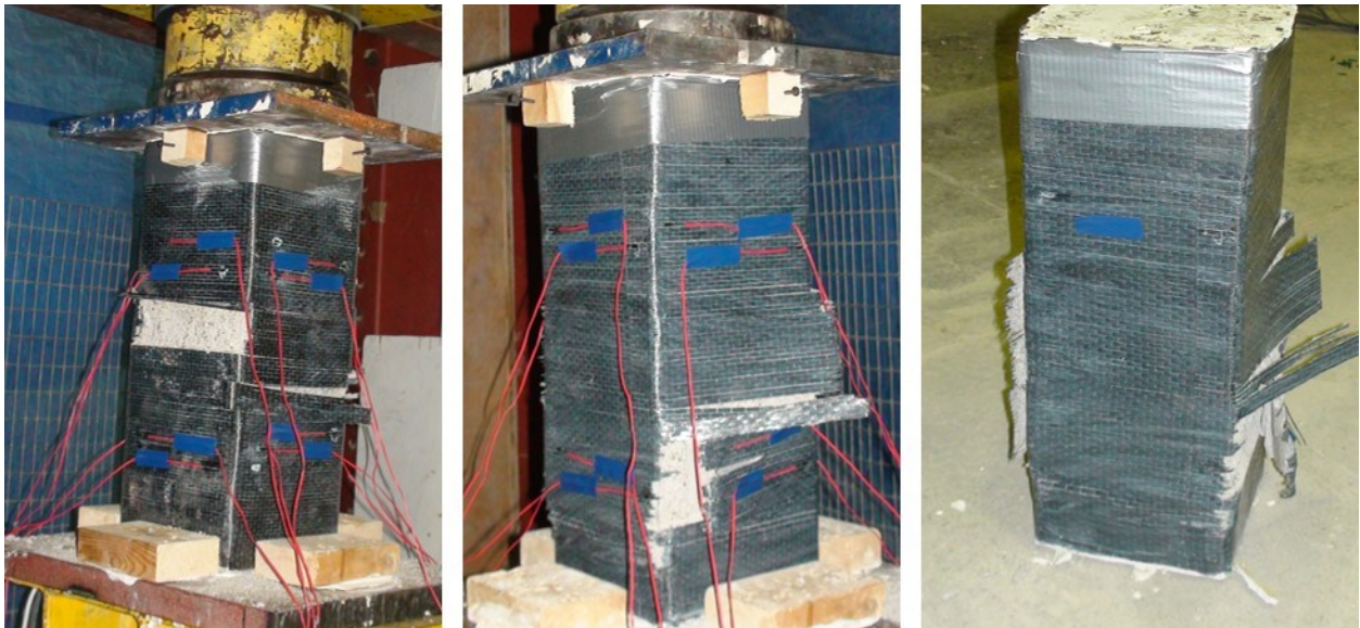
Figure C.4 Failure modes at the end of the compression tests for R10-L1.
