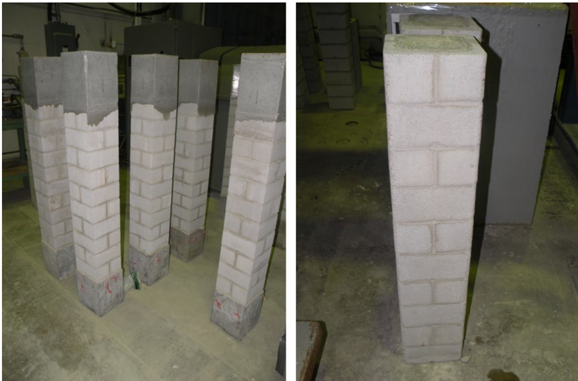
Figure A.22 Reinforced concrete masonry columns and ten course concrete masonry prisms.
