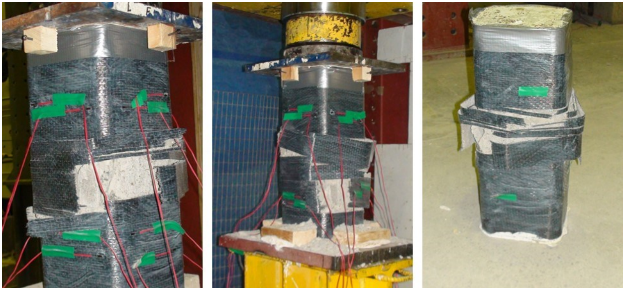
Figure C.14 Failure modes at the end of the compression tests for R30-L3.
