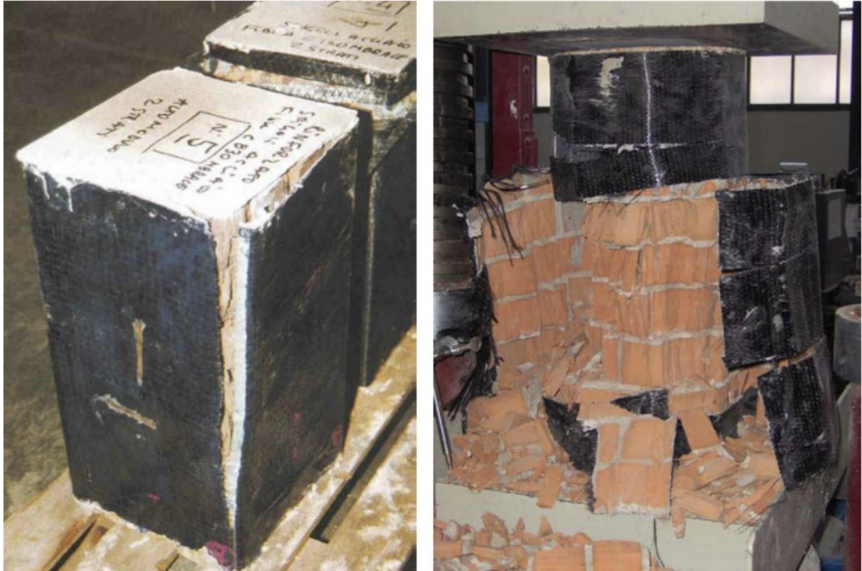
Figure 2.12 Failure of Square and octagonal cross section column (Corradi et al., 2007).
