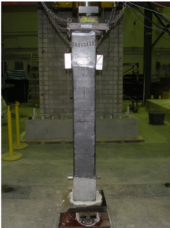
Figure A.30 Test setup for wrapped columns under eccentric load.
