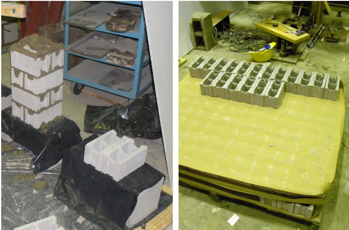
Figure A.1 Construction of concrete masonry prisms.
