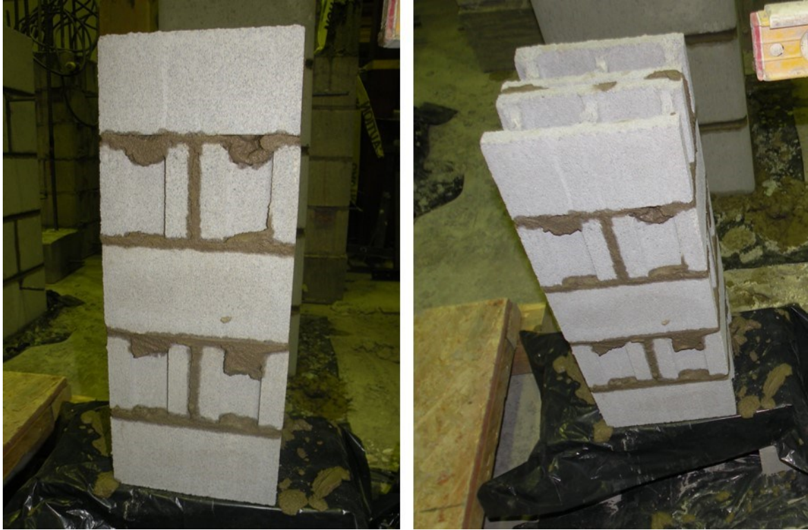
Figure A.2 UngROUTed concrete masonry prisms.
