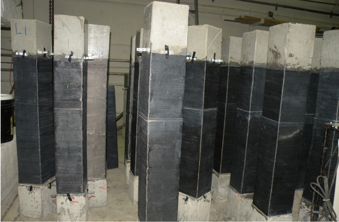
Figure A.23 Wrapped reinforced concrete masonry columns.
