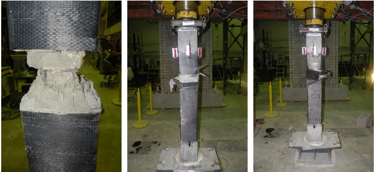
Figure C.20 Failure modes at the end of the compression tests for L2-e0.
