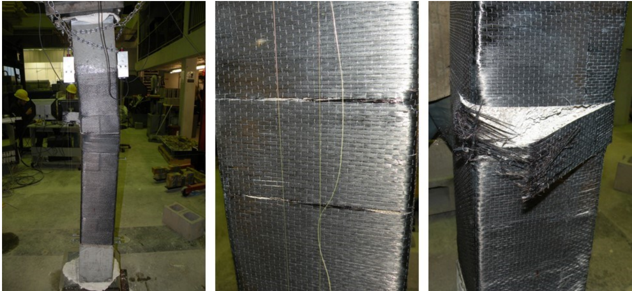
Figure C.30 Failure modes at the end of the eccentric tests for L2-e20.
