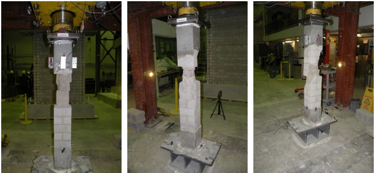
Figure C.16 Failure modes at the end of the compression tests for L0-e0.
