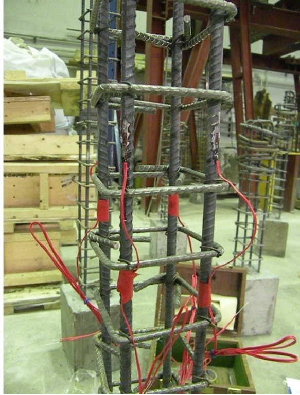
Figure A.19 Attaching strain gage to reinforcement steel.
