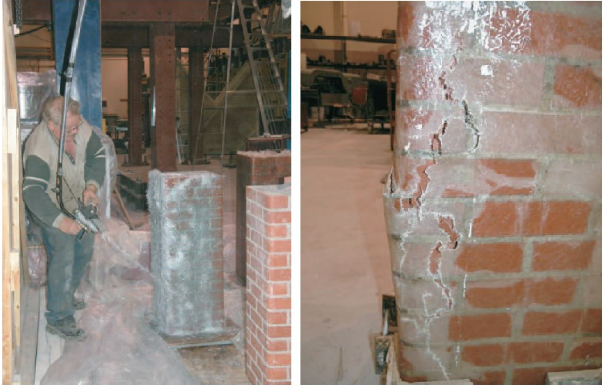
Figure 2.13 GFRP spray process and GFRP failure laminates (Shaheen and Shrive, 2007).
