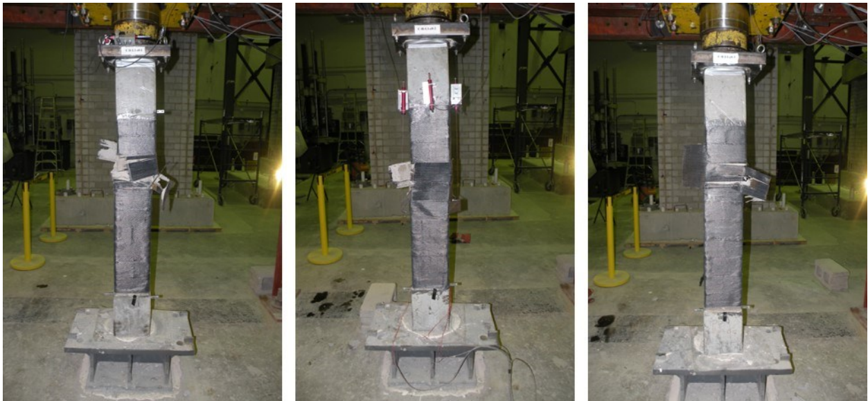
Figure C.18 Failure modes at the end of the compression tests for L1-e0.
