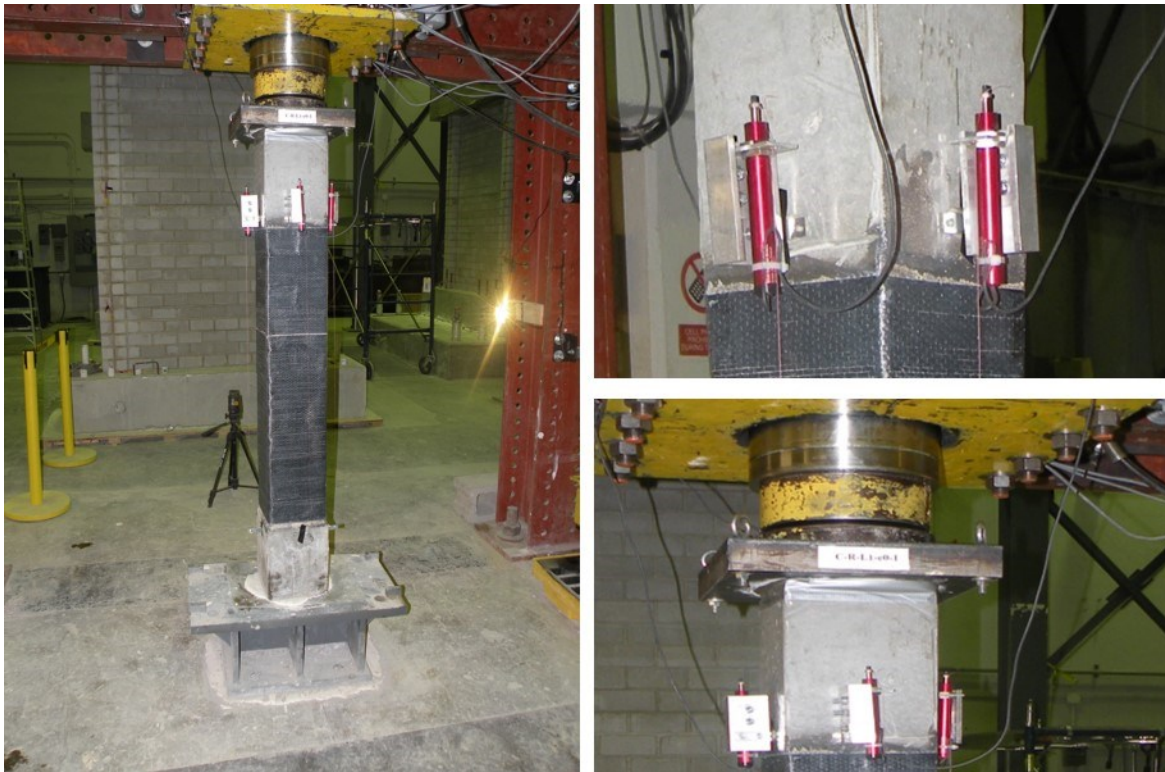
Figure A.28 Test setup for concentric load.
