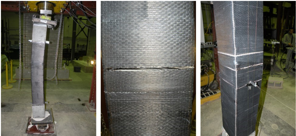
Figure C.32 Failure modes at the end of the eccentric tests for L2-e40.
