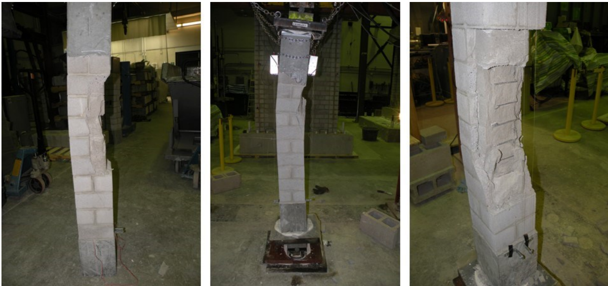
Figure C.22 Failure modes at the end of the eccentric tests for L0-e20.
