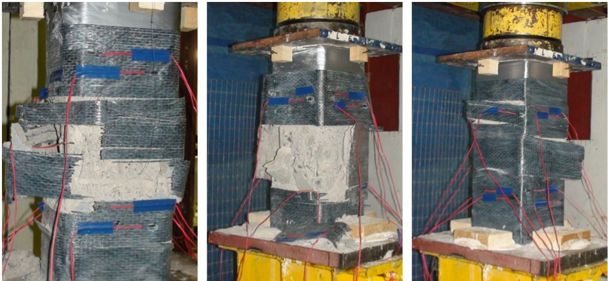
Figure C.12 Failure modes at the end of the compression tests for R30-L2.
