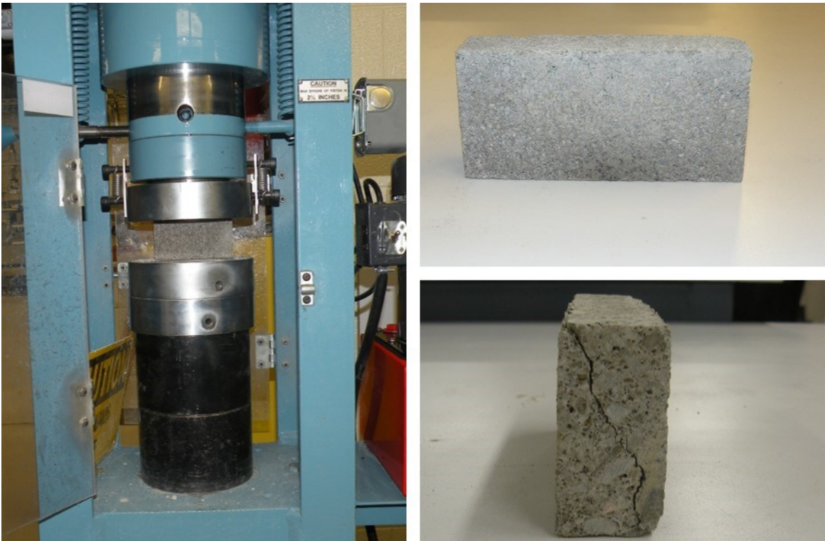
Figure A.24 Testing coupons of half-scale pilaster units.
