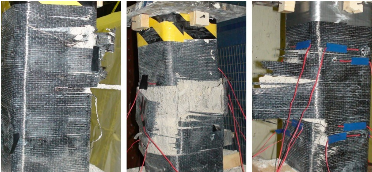
Figure C.10 Failure modes at the end of the compression tests for R30-L1.
