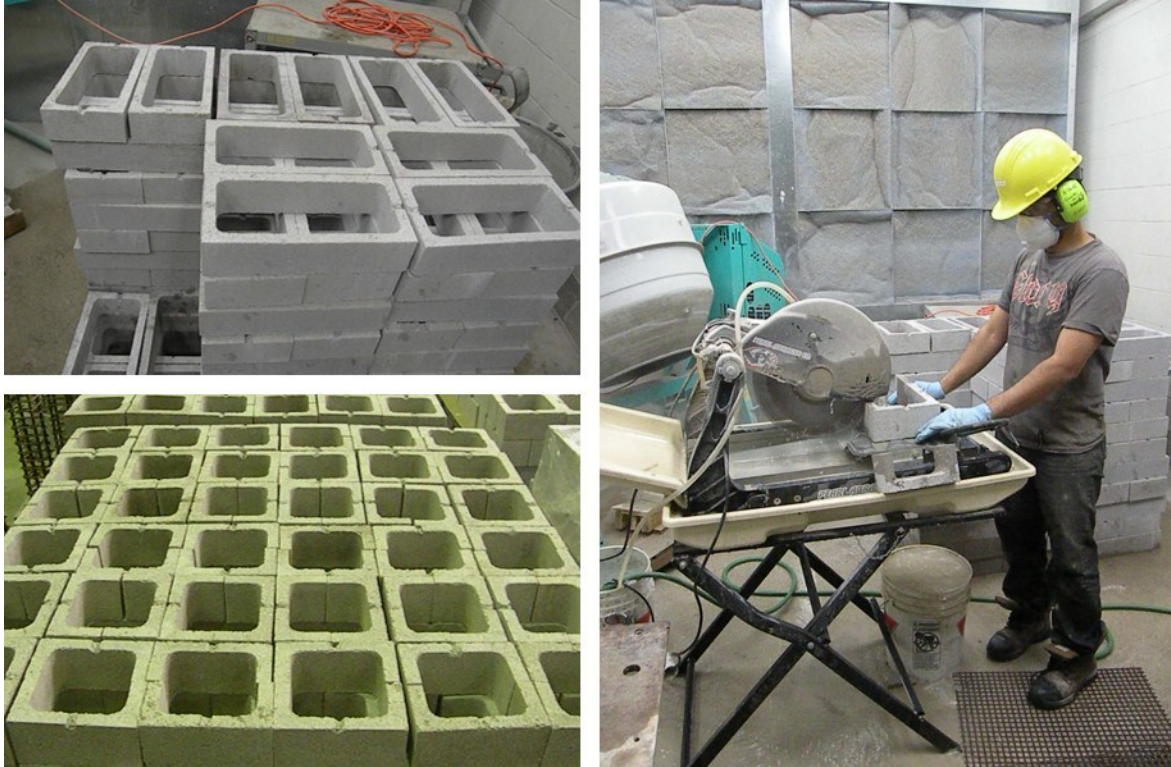
Figure A.17 Cutting half scale concrete masonry blocks.
