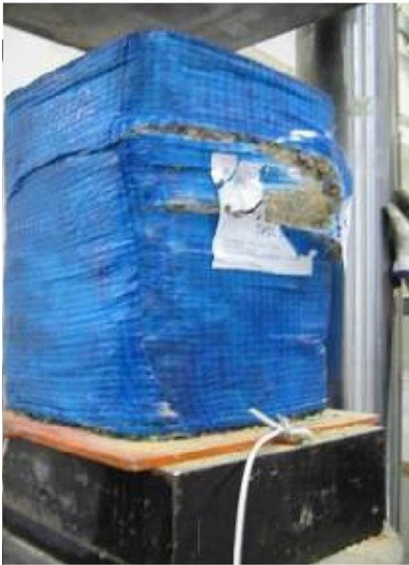
Figure 2.19 Failure of masonry columns with FRP composite (Faella et al., 2011b).
