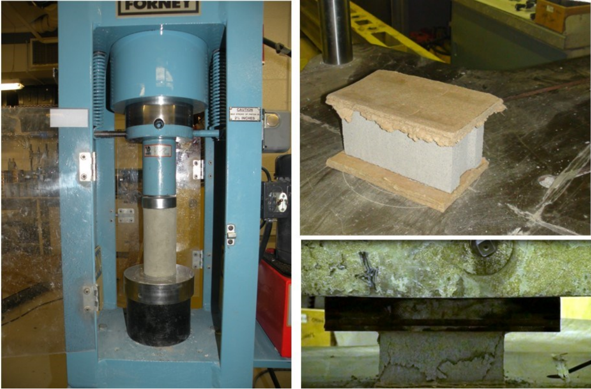
Figure A.5 Testing grout cylinder and half-scale block.
