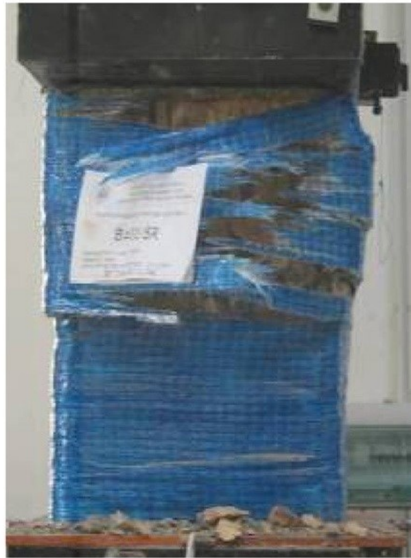
Figure 2.19 Failure of masonry columns with FRP composite (Faella et al., 2011b).
