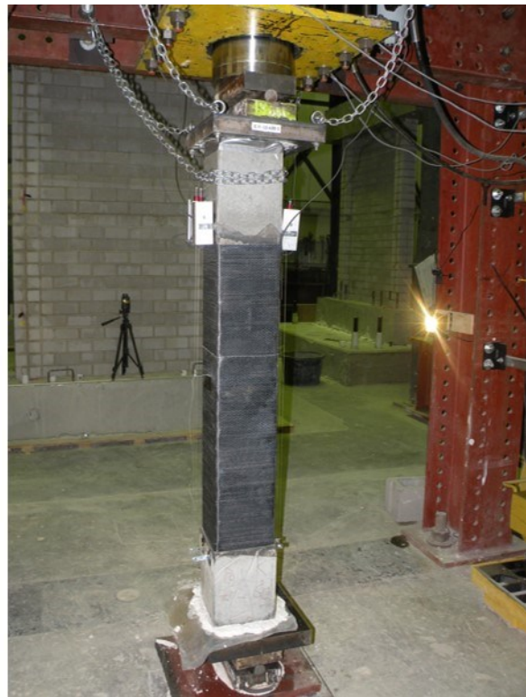
Figure A.30 Test setup for wrapped columns under eccentric load.
