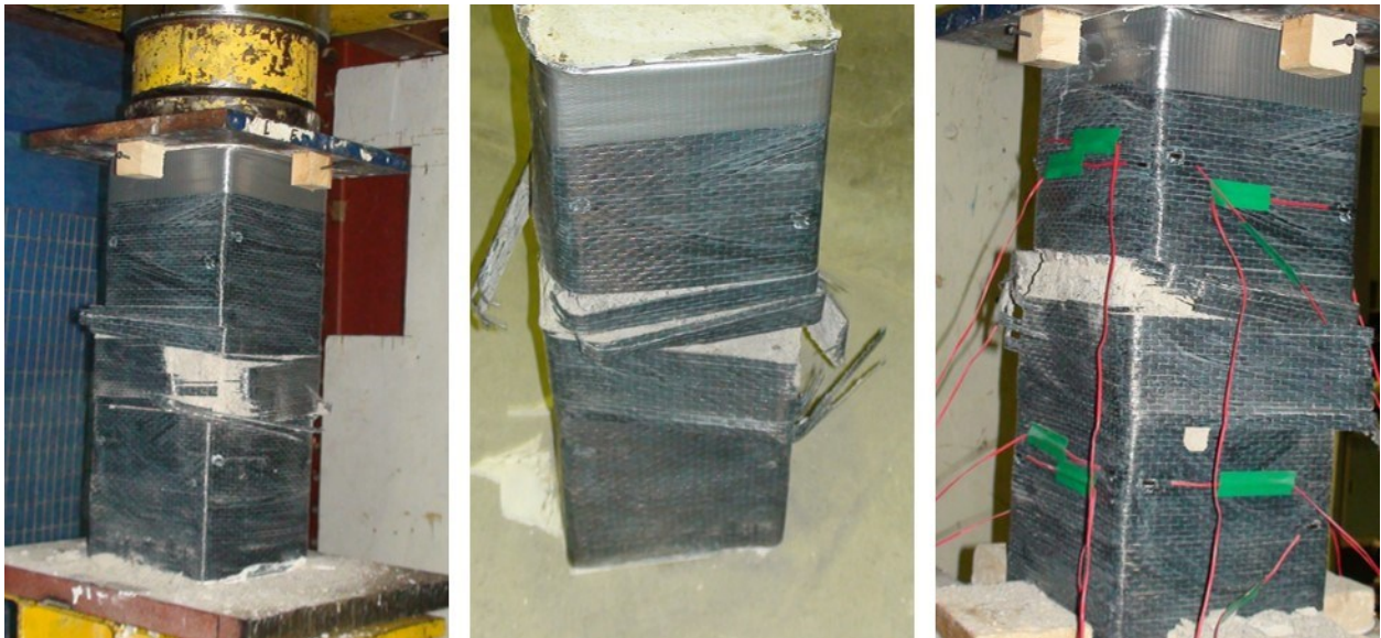
Figure C.8 Failure modes at the end of the compression tests for R10-L3.
