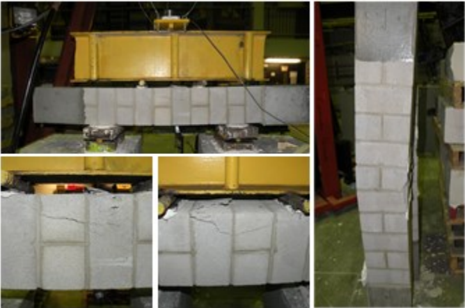
Figure 4.16 The failure mode of the beam at the end of the test.
