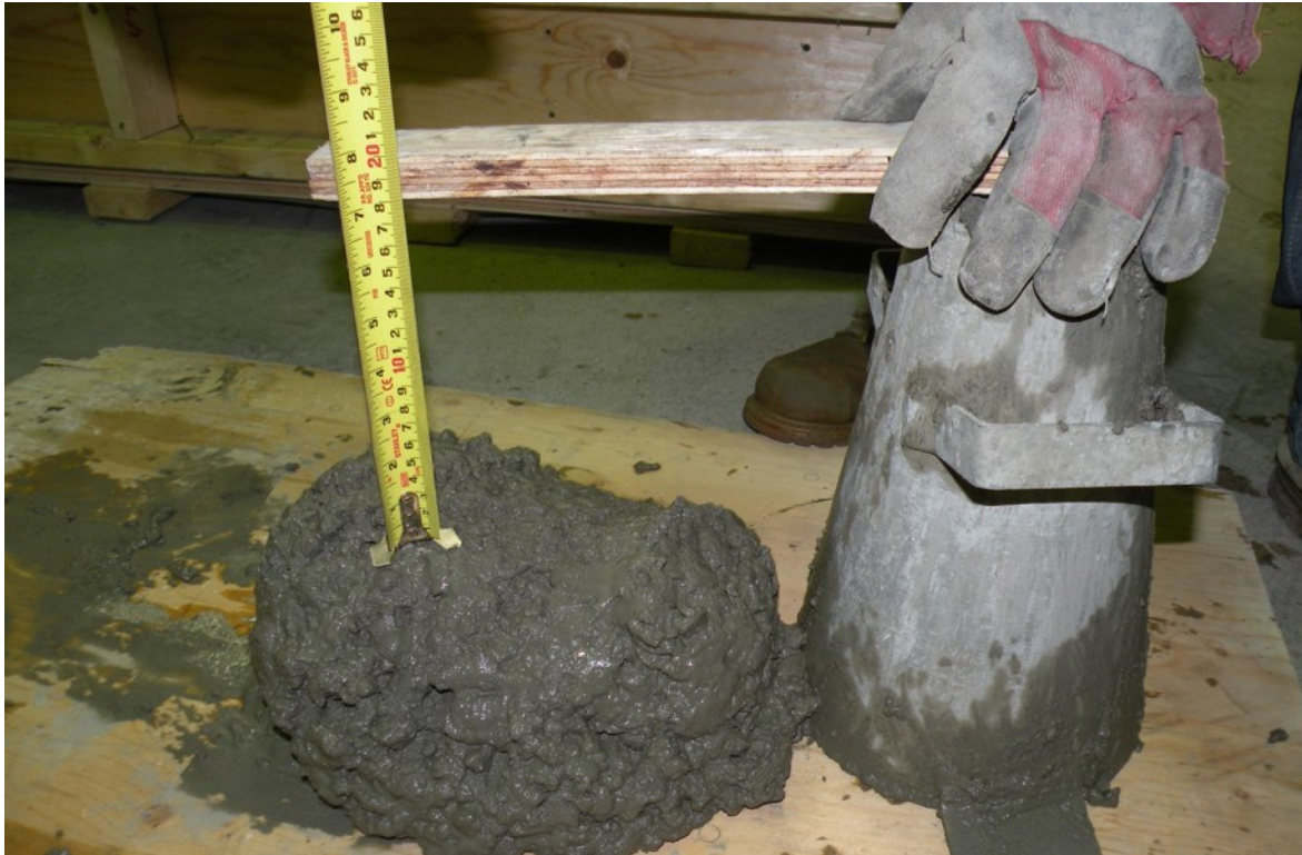
Figure A.27 Slump test.
