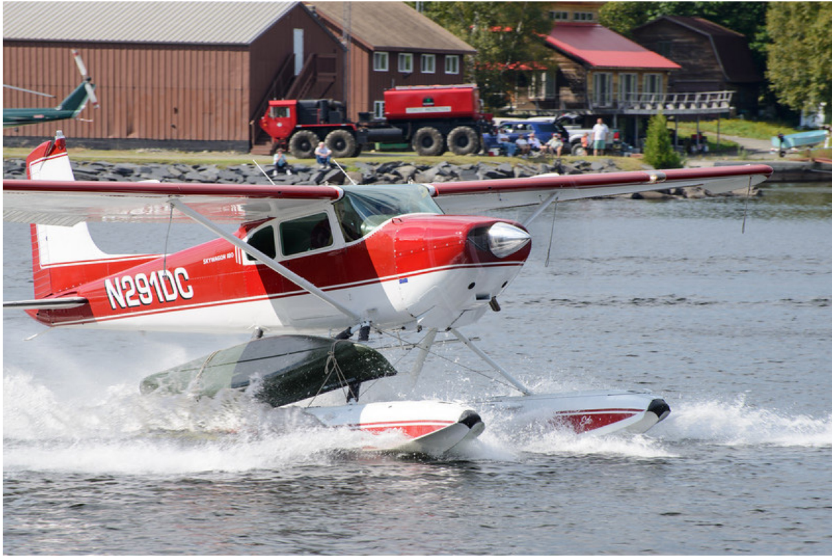
Figure 1: “Cessna 180 in the bush pilot canoe race”, demonstration of 1959-1963 Canoe-carrying capability STC for Cessna 180 [24]
