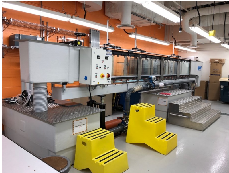
Figure 3-1: Experimental Flume in Water Resources Engineering Laboratory at Concordia University, used in the study.
