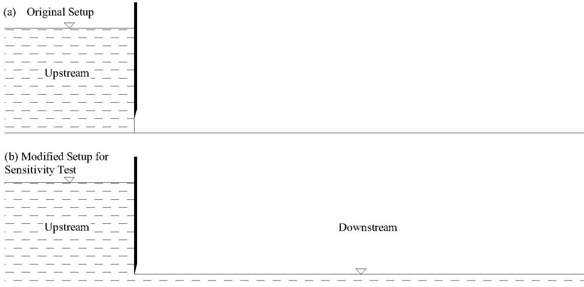
Figure 5-1: Sensitivity test of the choice of initial condition. a) the original setup for all of the simulations: the initial water position is placed before the sluice gate, with the desired flow depth, y_1 , b) the modified setup for the sensitivity test: the initial water position is placed before and after the sluice gate. On the upstream, the flow depth is set as y_1 ; on the downstream, the flow depth equals to the gate opening size.
