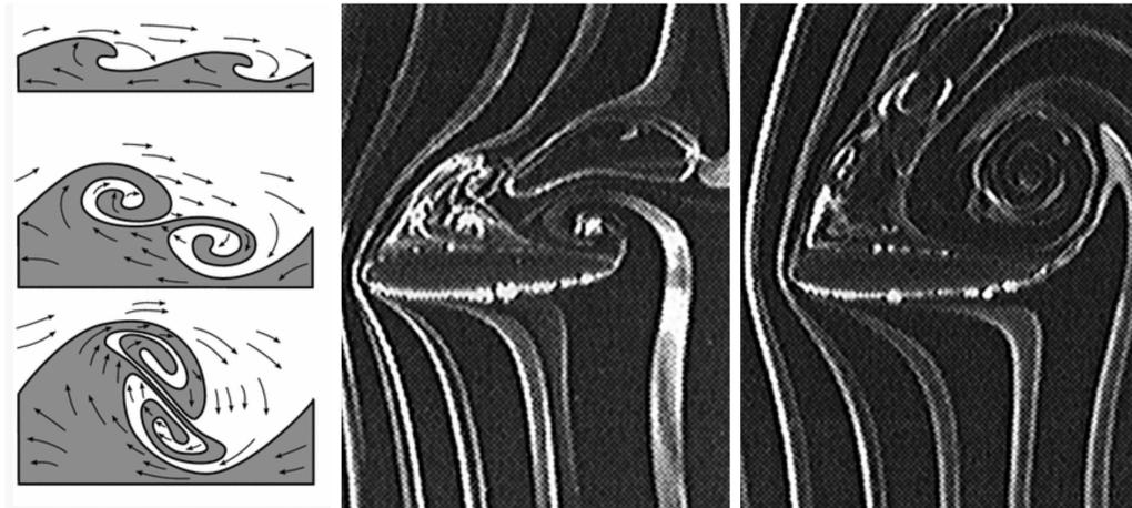
Figure 8: a drawing of the expected leading edge vortex roll-up, and images of the leading edge vortex roll-up from experiment [15] [23]
