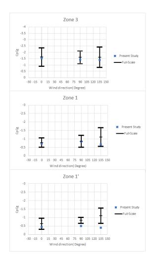
Figure 5-23: Comparison of peak pressure coefficients versus wind direction for zone 3, zone 1, and zone 1' between the results of the present study and the full-scale data measured on the experimental building of Duro-Last Roofing, Inc. in Iowa site.
