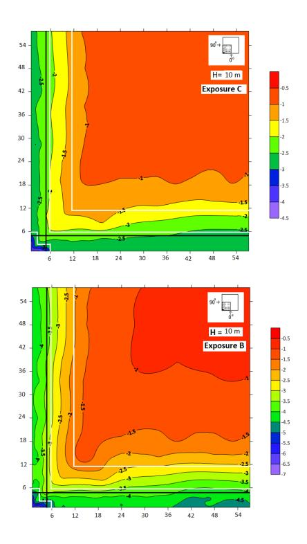
Figure 6-6: Contour of most critical peak pressure coefficients for the building of 10 m height in both exposure with the pressure zones of ASCE 7-16 (white lines) and NBCC 2015 and ASCE 7-10 (black
