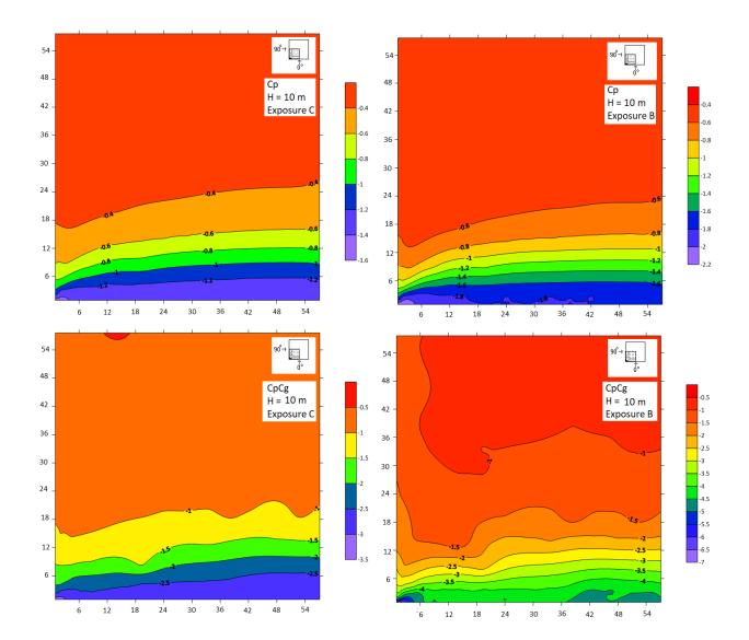
Appendix C 1: Contours of mean and peak pressure coefficients for 0° wind direction in exposure C and exposure B.
