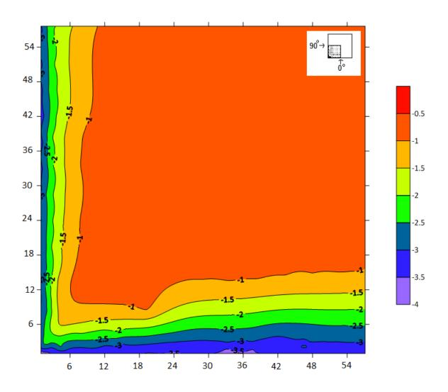
Figure 5-2: Values of most critical peak pressure coefficients (CpCg) for all wind directions (H=5 m, Exposure C).
