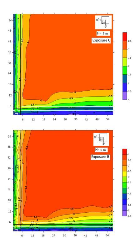
Figure 6-5: Contour of most critical peak pressure coefficients for the building of 5 m height in both exposure with the pressure zones of ASCE 7-16 (white lines) and NBCC 2015 and ASCE 7-10 (black
