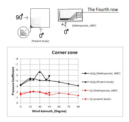
Figure 5-20: Comparison of extreme peak and mean pressure coefficients on the corner zone between the present study and Stathopoulos (1987).
