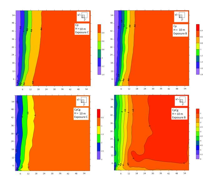
Appendix C 7: Contours of mean and peak pressure coefficients for 90° wind direction in exposure C and exposure B.
