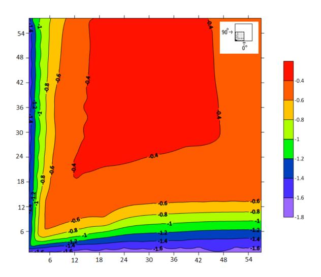
Figure 5-1: Values of most critical mean pressure coefficients (Cp) for all wind directions (H=5 m, Exposure C).
