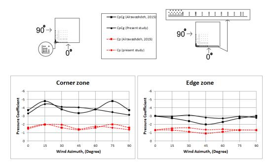
Figure 5-18: Comparison of extreme peak and mean pressure coefficients on the corner and the edge zones between the present study and Alrawashedeh and Stathopoulos, 2015.
