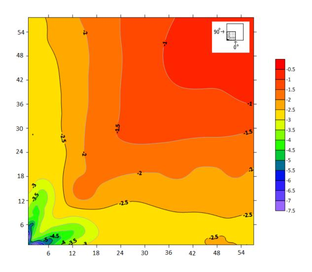
Figure 5-6: Values of most critical peak pressure coefficients (CpCg) for all wind directions (H=20 m., Exposure C).
