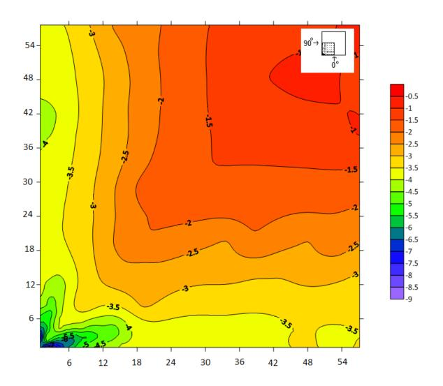
Figure 5-12: Values of most critical peak pressure coefficients (CpCg) for all wind directions (H=20 m, Exposure B).
