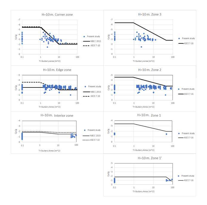
Figure 6-3: Comparison of the most critical area-averaged peak pressure coefficients, CpCg, of the present study and the values recommended by the codes (H=10 m, Exposure C).
