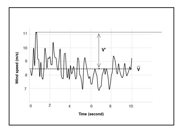
Figure 2-2: Wind speed recorded over a period of 10 seconds in the wind tunnel of Concordia University at height of 5 cm in the wind tunnel scale.
