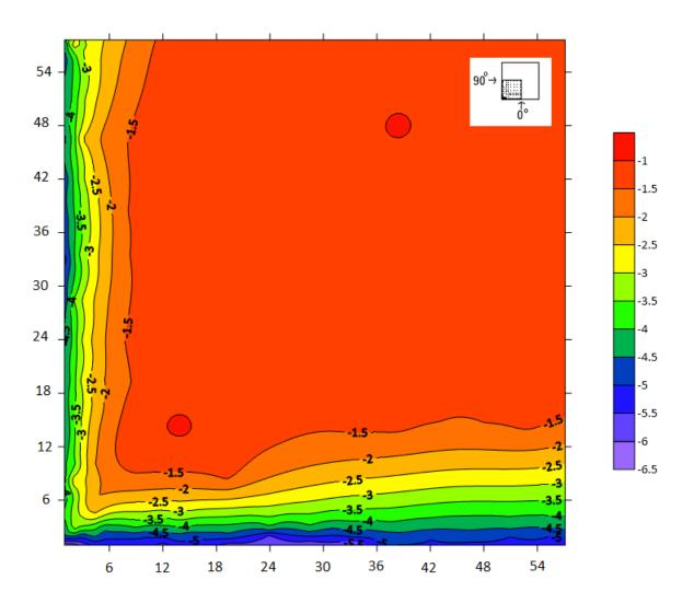
Figure 5-8: Values of most critical peak pressure coefficients (CpCg) for all wind directions (H=5 m, Exposure B).
