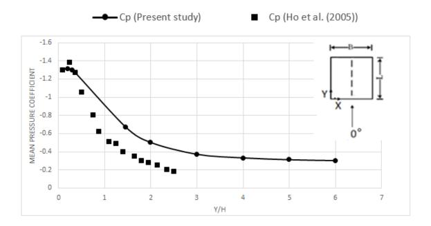
Figure 5-21: Variation of wind pressure coefficients of the present study and Ho et al (2005) along the roof centerline for normal wind direction.
