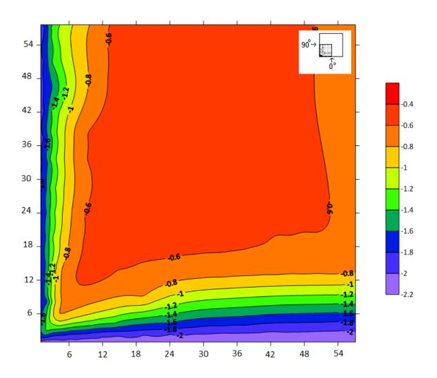
Figure 5-7: Values of most critical mean pressure coefficients (Cp) for all wind directions (H=5 m, Exposure B).
