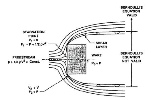
Figure 2-4: Flow around rectangular building, from Stathopoulos (2007).
