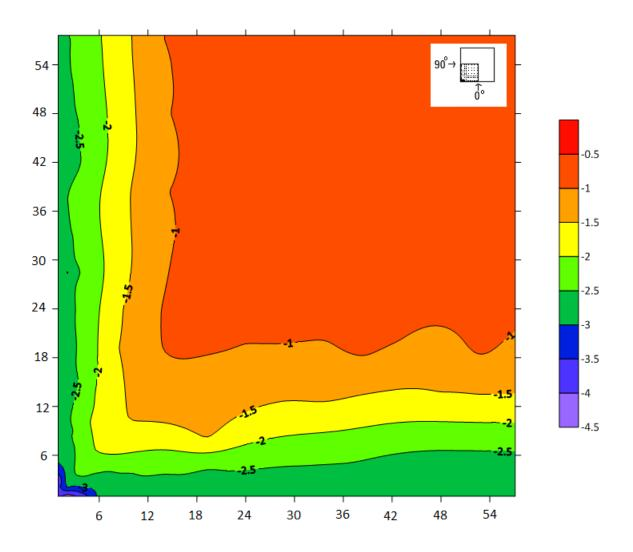
Figure 5-4: Values of most critical peak pressure coefficients (CpCg) for all wind directions (H=10 m, Exposure C).
