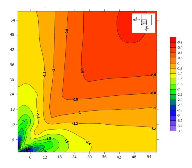
Figure 5-5: Values of most critical mean pressure coefficients (Cp) for all wind directions (H=20 m, Exposure C).
