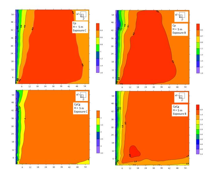
Appendix B 6: Contours of mean and peak pressure coefficients for 75° wind direction in exposure C and exposure B.
