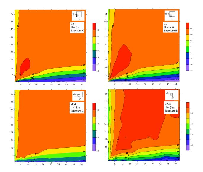
Appendix B 3: Contours of mean and peak pressure coefficients for 30° wind direction in exposure C and exposure B.
