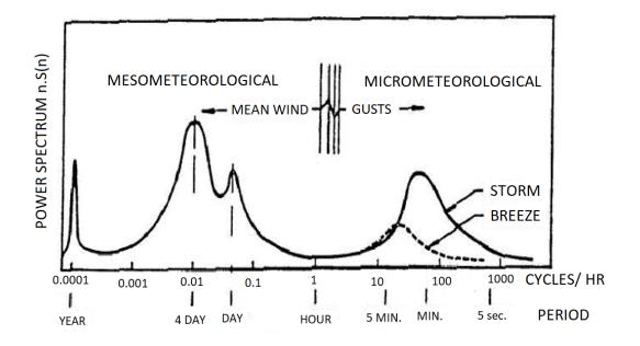
Figure 2-3: Wind spectrum after Van der Hoven (1957).
