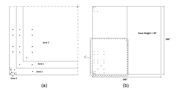
Figure 5-22: The experimental building of Duro-Last Roofing Inc. (a) Detailed pressure tap assembly, (b) Roof plan dimensions with pressure tap layout.
