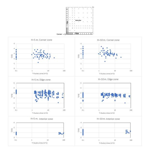
Figure 5-15: Most critical area-averaged peak pressure coefficients for all wind directions on the pressure zones defined by ASCE 7-10 and NBCC 2015 for buildings of 5 m and 10 m heights.
