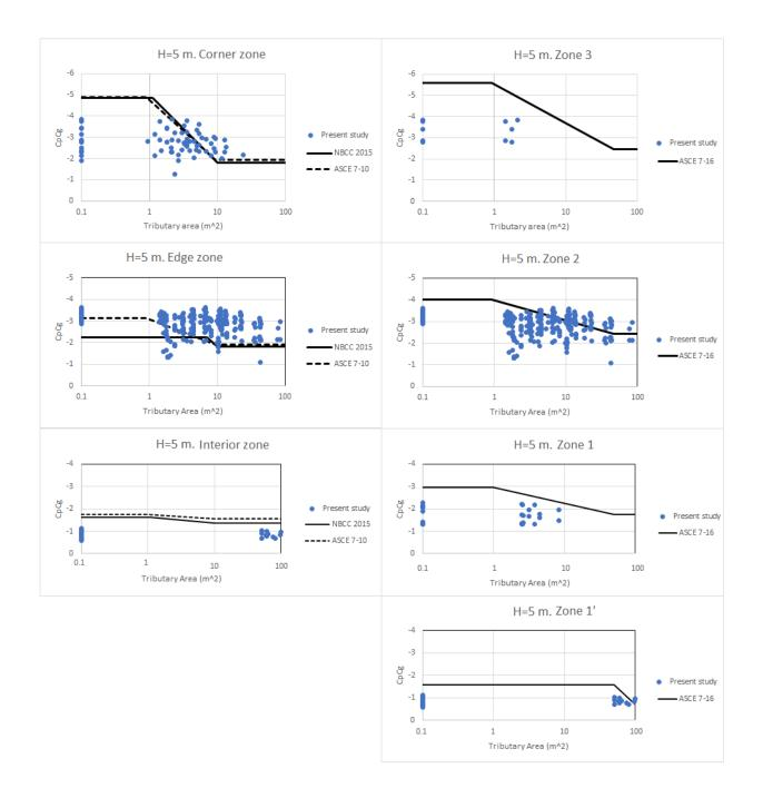
Figure 6-2: Comparison of the most critical area-averaged peak pressure coefficients, CpCg, of the present study and the values recommended by the codes (H=5 m, Exposure C).
