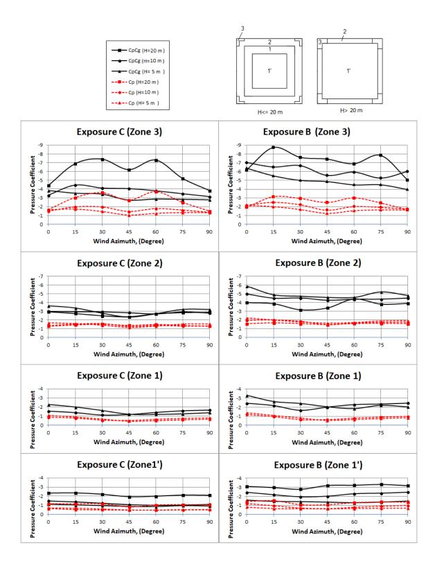
Figure 5-14: Extreme peak and mean pressure coefficients for pressure zones defined by ASCE 7-16 versus wind direction for 3 different heights and two exposures.
