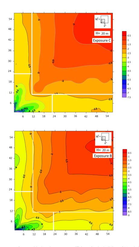
Figure 6-7: Contour of most critical peak pressure coefficients for the building of 20 m height in both exposures with the pressure zones of ASCE 7-16, NBCC 2015 and ASCE 7-10.
