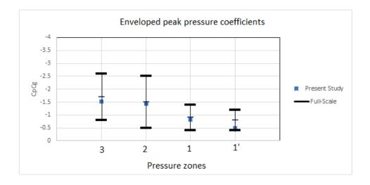
Figure 5-24: Comparison of the enveloped peak pressure coefficients between the full-scale data and the present study in ASCE 7 roof pressure zones.
