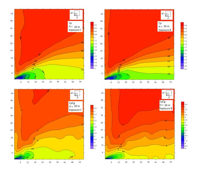
Appendix D 2: Contours of mean and peak pressure coefficients for 15° wind direction in exposure C and exposure B.
