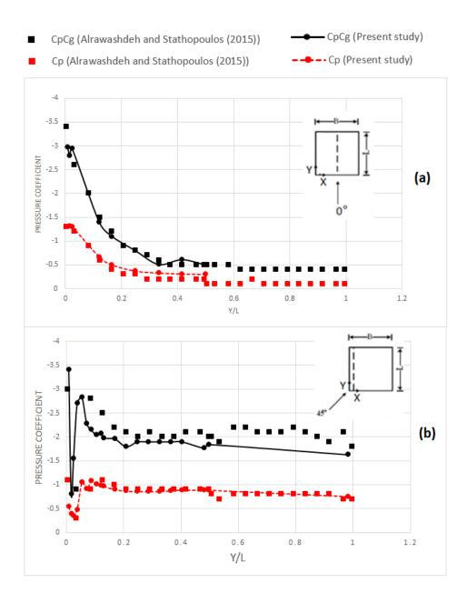
Figure 5-19: Comparison between the present study and Alrawashdeh and Stathopoulos (2015), a) Variation of wind pressure coefficients along the roof centerline for  $0^{\circ}$  wind direction; b) Variation in wind pressure coefficients along the line at the concurrent edge for  $45^{\circ}$  wind direction.
