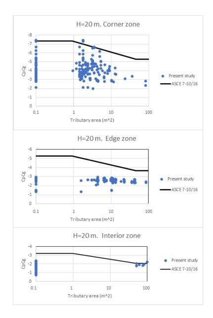
Figure 6-4: Comparison of the most critical area-averaged peak pressure coefficients, CpCg, of the present study and the values recommended by ASCE 7-10/16 (H=20 m, Exposure C).
