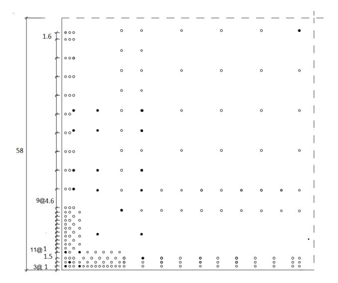
Figure 4-6: Detailed pressure tap assembly in the bottom-left quarter of the roof (dimensions in meter).
