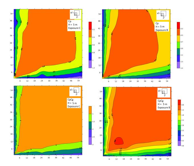
Appendix B 4: Contours of mean and peak pressure coefficients for 45° wind direction in exposure C and exposure B.
