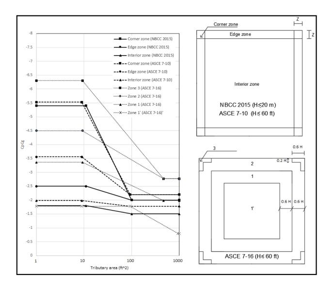
Figure 3-2: External peak pressure coefficients (NBCC format) of the North American codes and standards for low-slope roofs of low-rise buildings (H  $\leq$  18 m).
