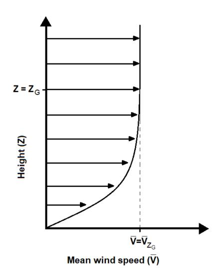
Figure 2-1: Vertical wind speed profile in the atmospheric boundary layer.
