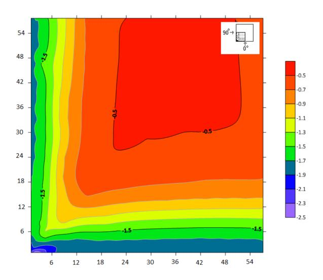
Figure 5-9: Values of most critical mean pressure coefficients (Cp) for all wind directions (H=10 m, Exposure B).
