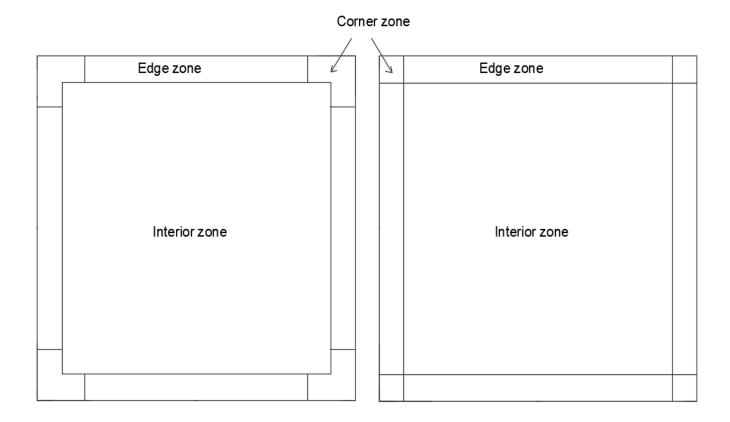
Figure 2-5: Roof pressure zones.
