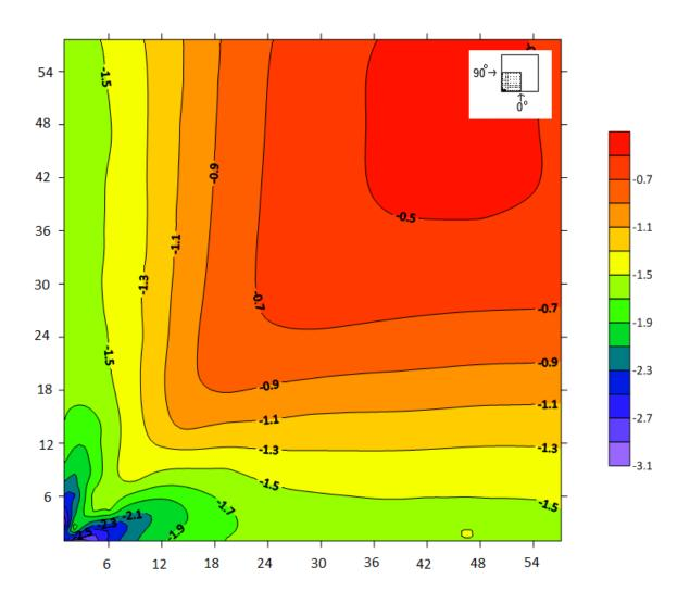
Figure 5-11: Values of most critical mean pressure coefficients (Cp) for all wind directions (H=20 m, Exposure B).
