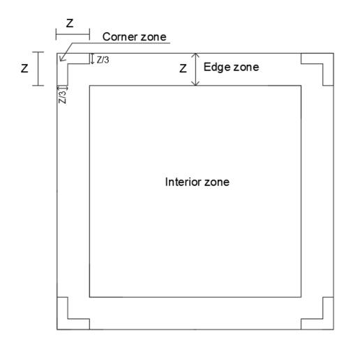
Figure 6-8: Proposed zonal system for low-slope low-rise buildings of heights more than 8 m and large geometries, z is the end-zone width defined in NBCC 2015.
