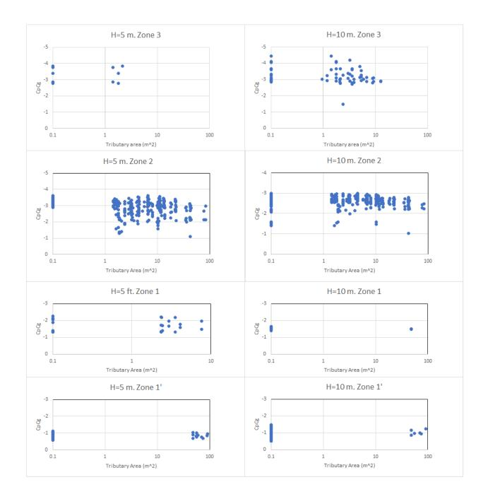
Figure 5-16: Most critical area-averaged peak pressure coefficients for all wind directions on the pressure zones defined by ASCE 7-16 for buildings of 5 m and 10 m heights.
