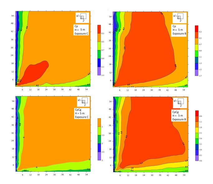
Appendix B 5: Contours of mean and peak pressure coefficients for 60° wind direction in exposure C and exposure B.
