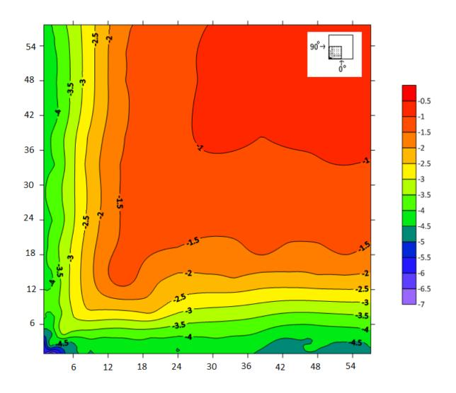
Figure 5-10: Values of most critical peak pressure coefficients (CpCg) for all wind directions (H=10 m, Exposure B).
