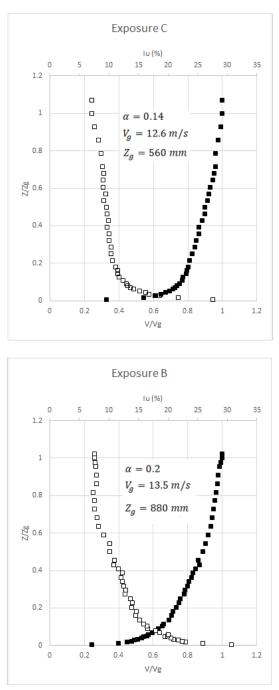
Figure 4-2: Vertical variation of mean wind speed and longitudinal turbulence intensity for exposure C
