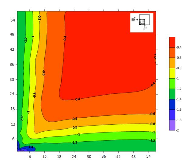
Figure 5-3: Values of most critical mean pressure coefficients (Cp) for all wind directions (H=10 m, Exposure C).
