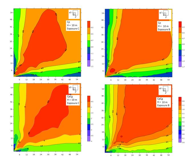
Appendix C 4: Contours of mean and peak pressure coefficients for 45° wind direction in exposure C and exposure B.
