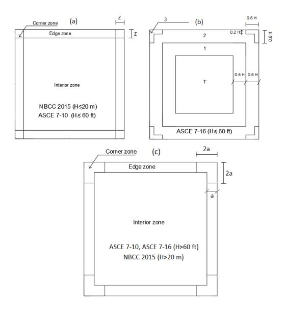
Figure 3-1: Roof zonal systems for low-slope roofs of low-rise and mid-rise buildings in the North American codes: (a) low-rise building in NBCC 2015 and ASCE 7-10, (b) low-rise building in ASCE 7-16 and (c) mid-rise building in the three codes.
