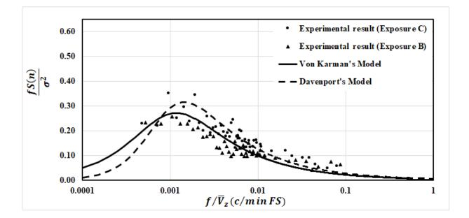
Figure 4-3: Power spectral density of longitudinal turbulence component evaluated at one-sixth the gradient height.
