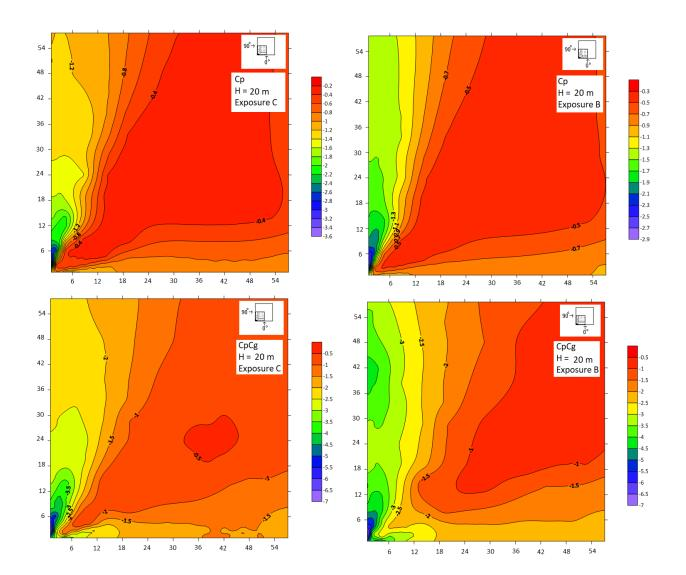
Appendix D 5: Contours of mean and peak pressure coefficients for 60° wind direction in exposure C and exposure B.
