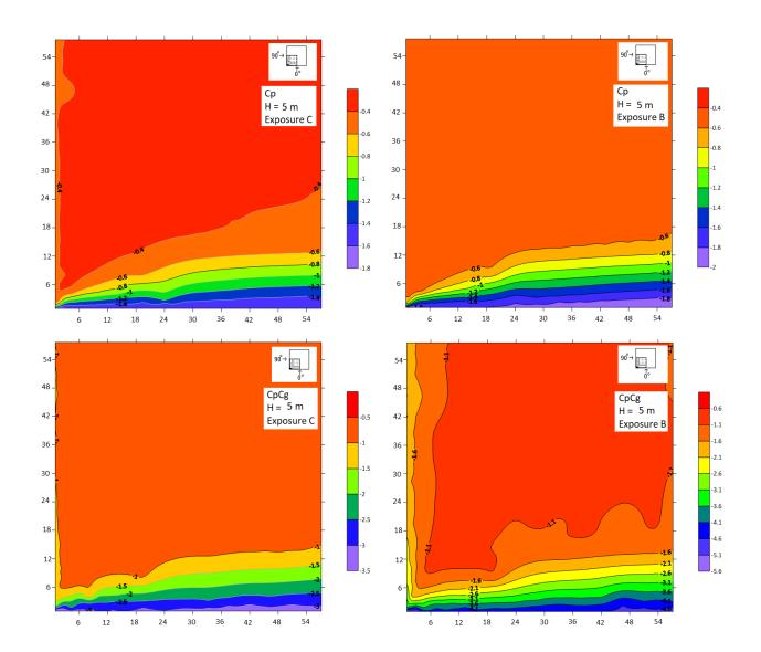
Appendix B 2: Contours of mean and peak pressure coefficients for 15° wind direction in exposure C and exposure B.
