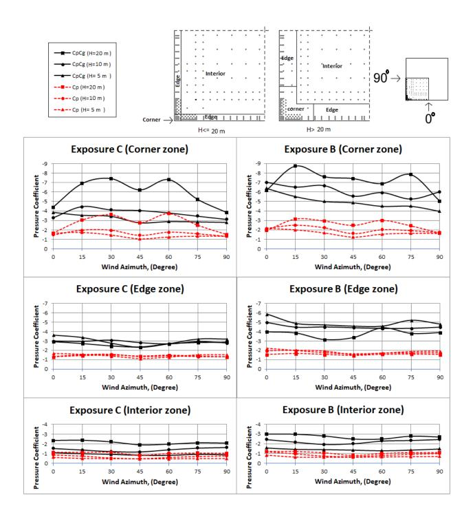
Figure 5-13: Extreme peak and mean pressure coefficients for pressure zones defined by ASCE 7-10 and NBCC 2015 versus wind direction for 3 different heights and two exposures.
