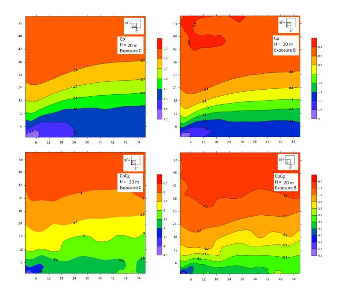
Appendix D 1: Contours of mean and peak pressure coefficients for 0° wind direction in exposure C and exposure B.
