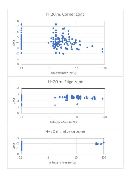
Figure 5-17: Most critical area-averaged peak pressure coefficients for all wind directions on pressure zones defined by NBCC 2015, ASCE 7-10 and ASCE 7-16 for building of 20 m height.
