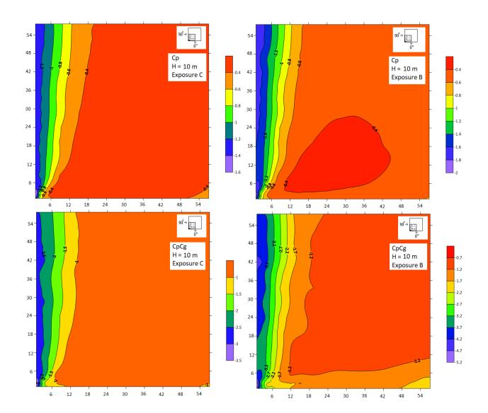
Appendix C 6: Contours of mean and peak pressure coefficients for 75° wind direction in exposure C and exposure B.
