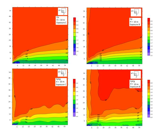
Appendix C 2: Contours of mean and peak pressure coefficients for 15° wind direction in exposure C and exposure B.
