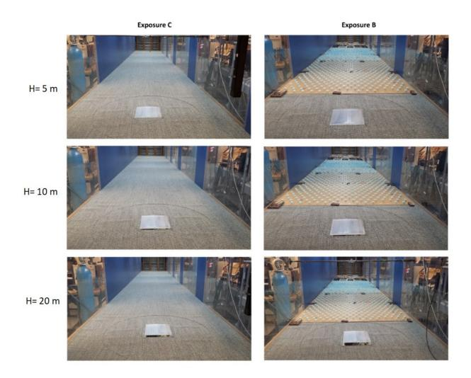
Figure 4-4: Installation of building models in the wind tunnel for both exposures.
