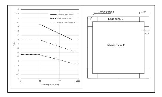
Figure 3-3: External peak pressure coefficients (NBCC format) of the ASCE 7-10 and ASCE 7-16 for roofs of mid-rise buildings.
