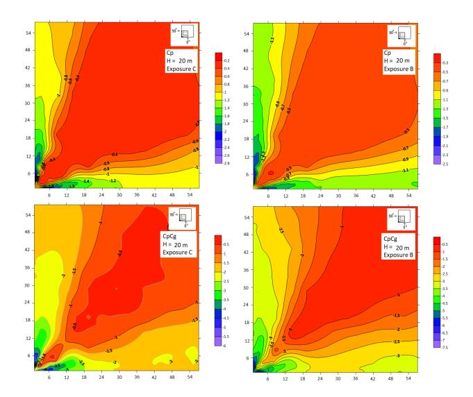
Appendix D 4: Contours of mean and peak pressure coefficients for 45° wind direction in exposure C and exposure B.
