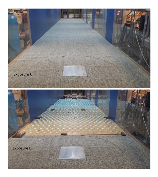
Figure 4-1: Simulation of exposure C and exposure B at the wind tunnel of Concordia University.
