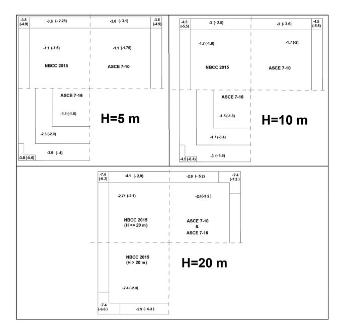
Figure 6-1: Comparison of most critical peak pressure coefficients between the present study for the three buildings in open country exposure and the corresponding recommended peaks of NBCC 2015, ASCE 7-10 and ASCE 7-16. (coefficients between brackets are the recommended codes values).
