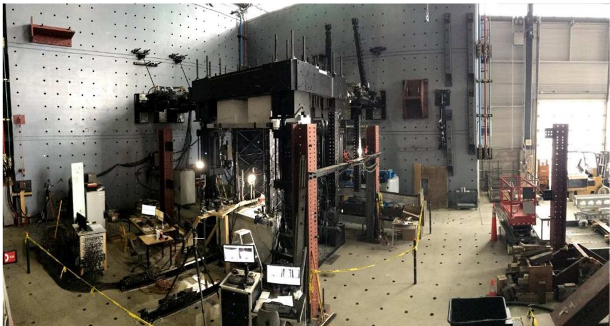
Fig. 6.17. General view of the 6DOF system at École Polytechnique's structures lab and the test setup of the FRP Retrofitted wall
