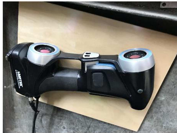
Fig. 6.23. 3D Encoders used for measuring the relative deformations in the 6DOF system
