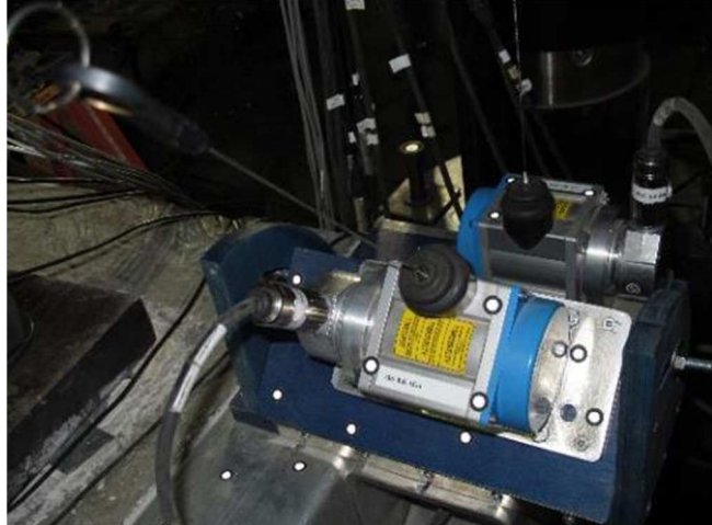
Fig. 6.23. 3D Encoders used for measuring the relative deformations in the 6DOF system
