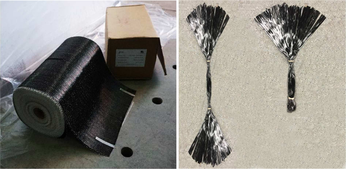
Fig. 6.14. FRP roll (Tyfo SCH 11UP) and FRP anchor (Tyfo SCH Composite Anchors)
