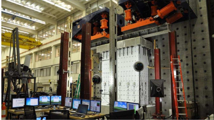
Fig. 2.7. Experimental tests on C-shaped RC walls (Lowes et al., 2013)
