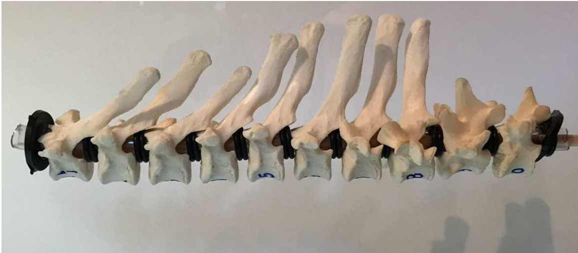
Figure 12: Canine vertebrae, with the vinyl tubing inserted through the cavities and the rubber O-rings between each vertebrae, prior to complete immersion into the gel.
