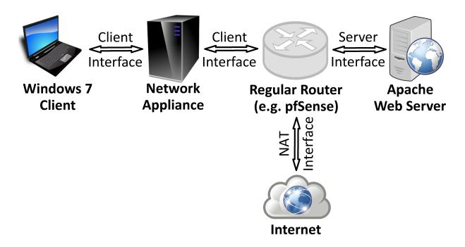
Figure 3.2: Framework components and test architecture with a router
