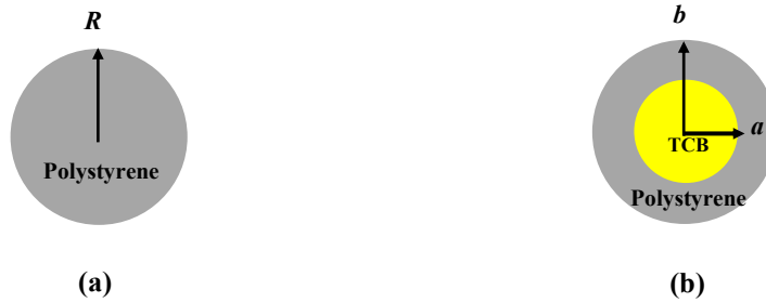
Figure 3.1. Schematics of samples used in rheological characterization of: (a) Neat polystyrene; (b) Solvent diffusion. The inner radius is variable, and two different geometries are studied.
